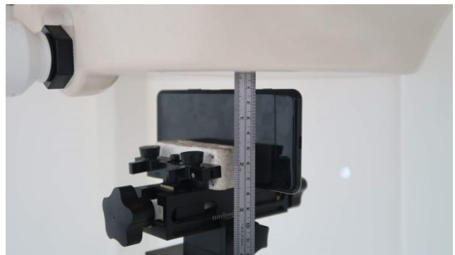
Right Side, Test Separation 10 mm
