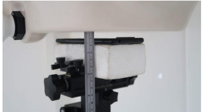
Back, Test Separation 10 mm
