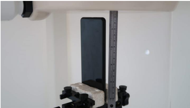
Bottom Side, Test Separation 10 mm
