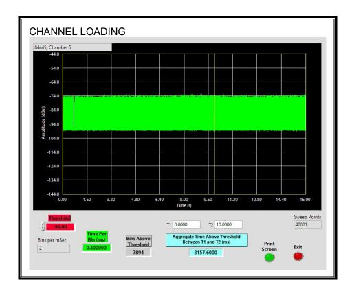
The level of traffic loading on the channel by the EUT is 31.58%
