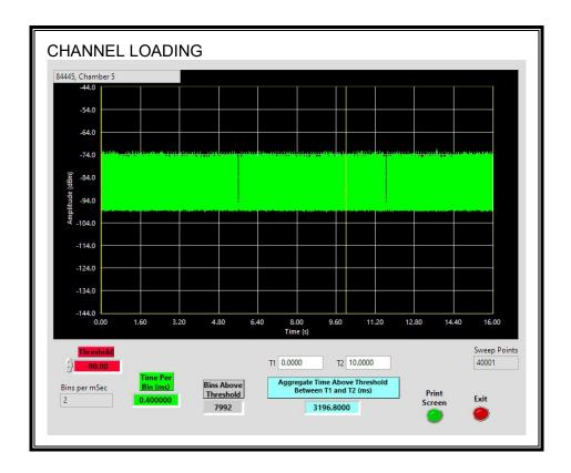
The level of traffic loading on the channel by the EUT is 31.97%
