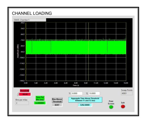
The level of traffic loading on the channel by the EUT is 32.83%
