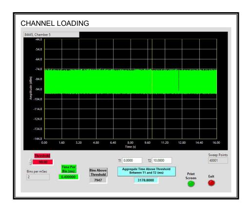
The level of traffic loading on the channel by the EUT is 31.79%
