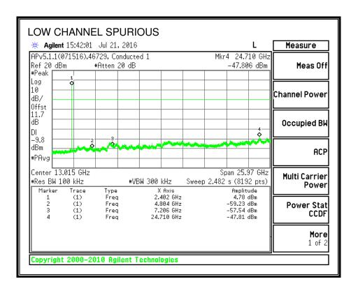
Note: Limit line should be -10.37 dBm, however margin is sufficient to be compliant.
