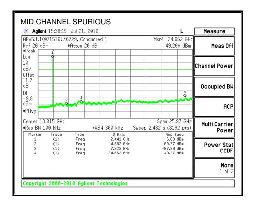
Note: Limit line should be -10.37 dBm, however margin is sufficient to be compliant.
