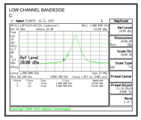
Note: Limit line should be -10.37 dBm, however margin is sufficient to be compliant.
