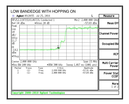
Note: Limit line should be -14.62 dBm, however margin is sufficient to be compliant.
