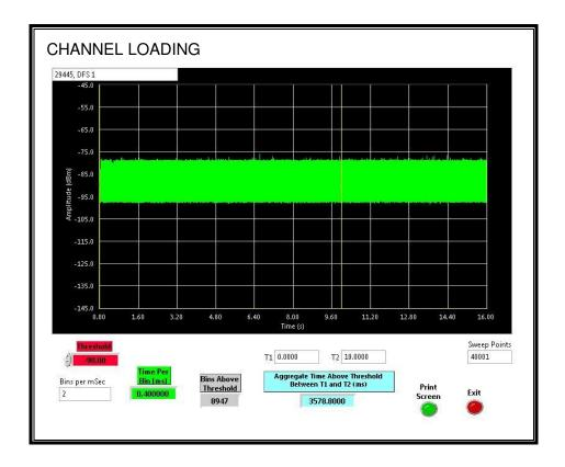
The level of traffic loading on the channel by the EUT is 35.78%
