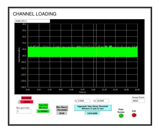
The level of traffic loading on the channel by the EUT is 34.19%
