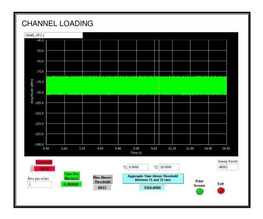
The level of traffic loading on the channel by the EUT is 35.68%
