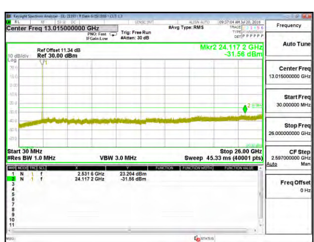
LTE B7 10MHz 16QAM Middle Channel
