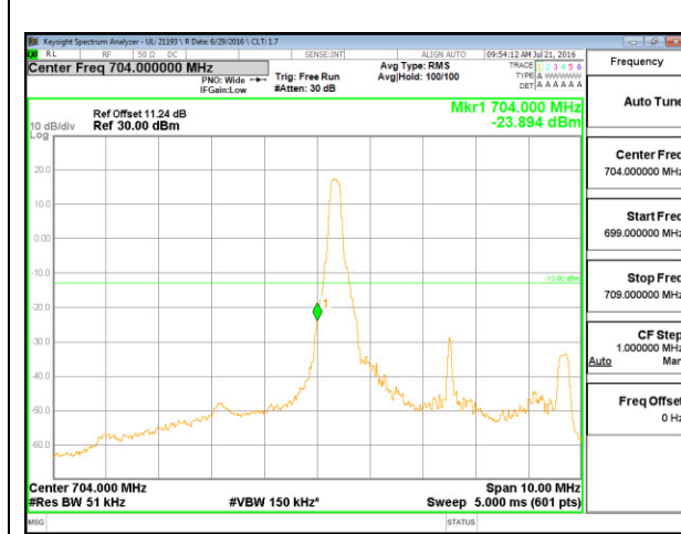
LTE B17 5MHz QPSK Low Channel 1RB
