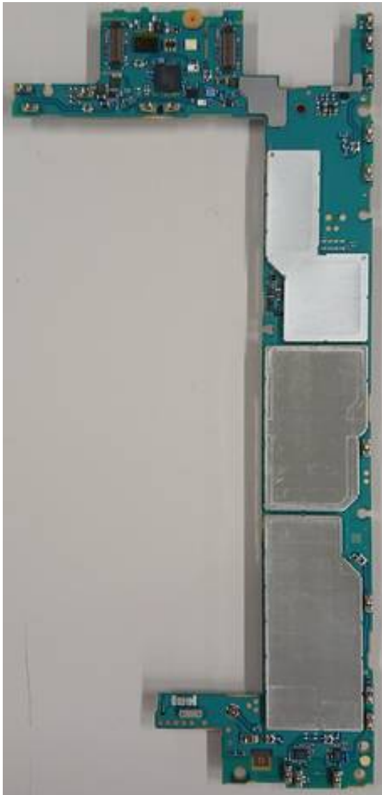
Internal PWB with Shield cases (Rear-side)
