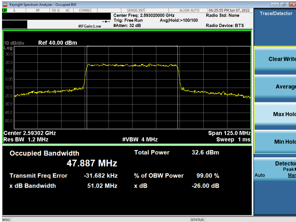
Plot 7-22. Occupied Bandwidth Plot (NR Band n41 - 50MHz QPSK - Full RB)
