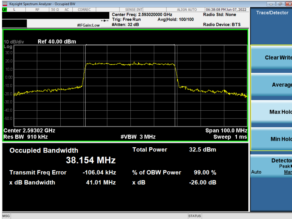
Plot 7-25. Occupied Bandwidth Plot (NR Band n41 - 40MHz QPSK - Full RB)
