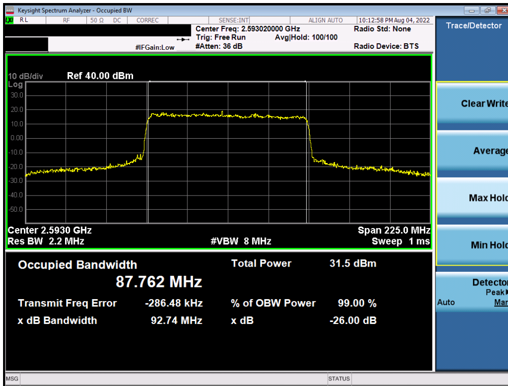
Plot 7-36. Occupied Bandwidth Plot (NR Band n41 - 90MHz 16-QAM - Full RB - Sub ANT)
