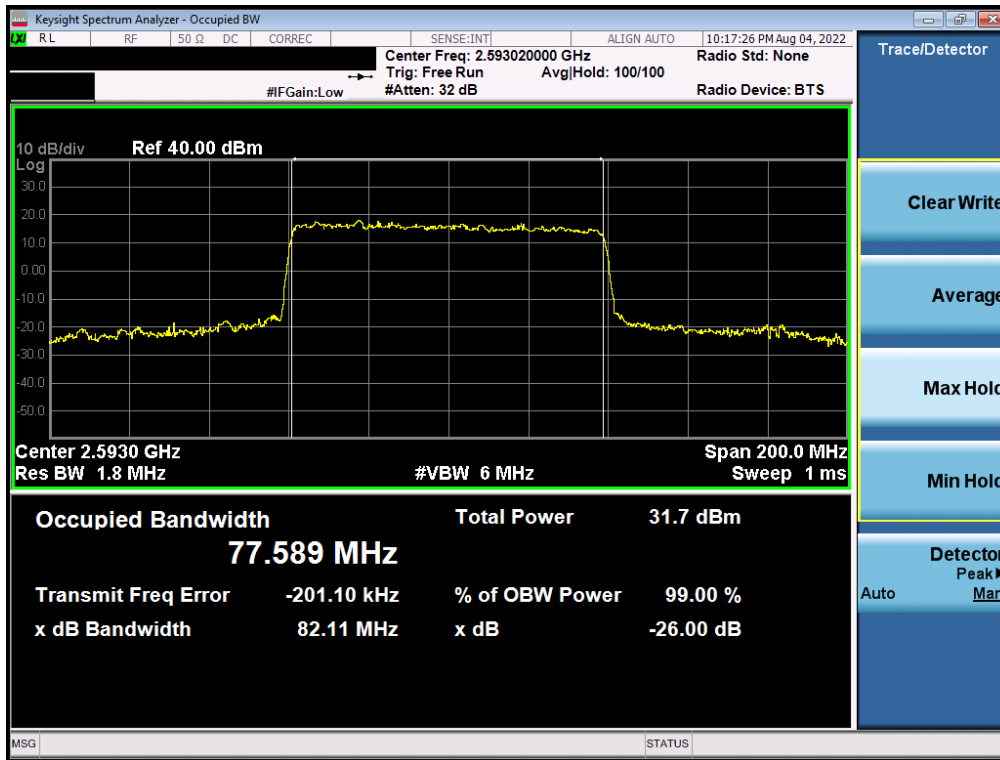
Plot 7-38. Occupied Bandwidth Plot (NR Band n41 - 80MHz 16-QAM - Full RB - Sub ANT)
