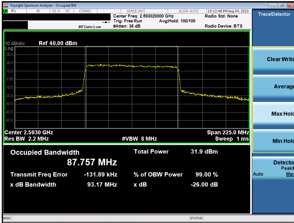
Plot 7-35. Occupied Bandwidth Plot (NR Band n41 - 90MHz QPSK - Full RB - Sub ANT)
