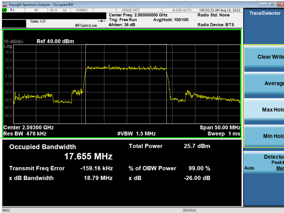
Plot 7-2. Occupied Bandwidth Plot (LTE Band 41(PC3) - 20MHz 16-QAM - Full RB)
