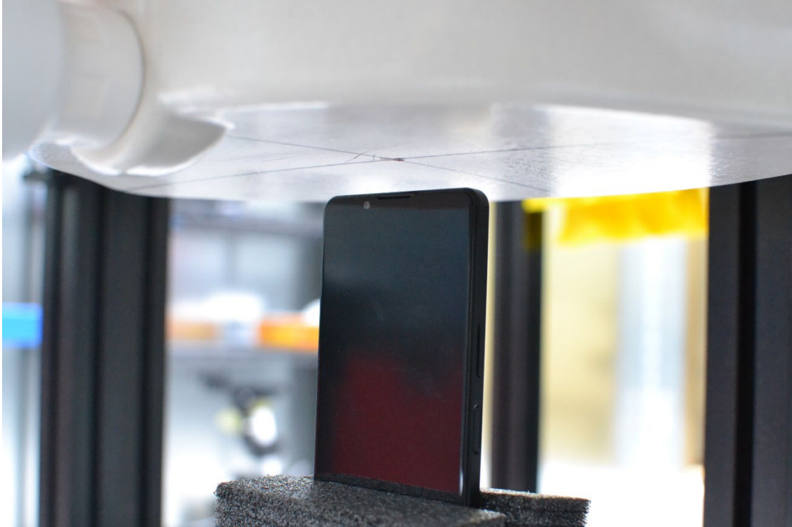
SAR Test Setup Photo 11 – Hotspot, Top Edge at 10mm
