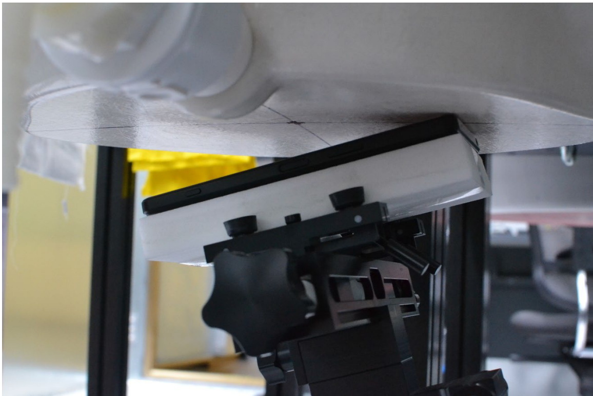
SAR Test Setup Photo 6 – Head, Left Cheek, Mouth Jaw for NR Band 77 and LTE Band 48 at 0mm
