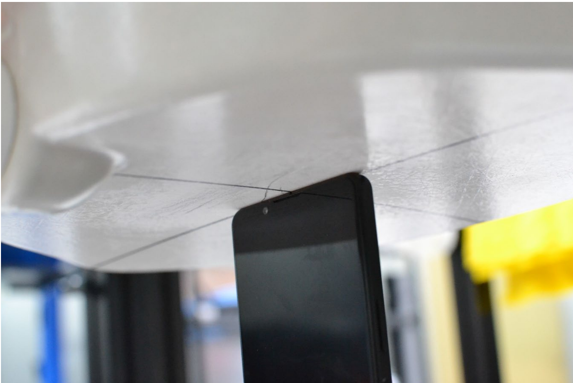
SAR Test Setup Photo 16 – Phablet, Top Side at 0mm
