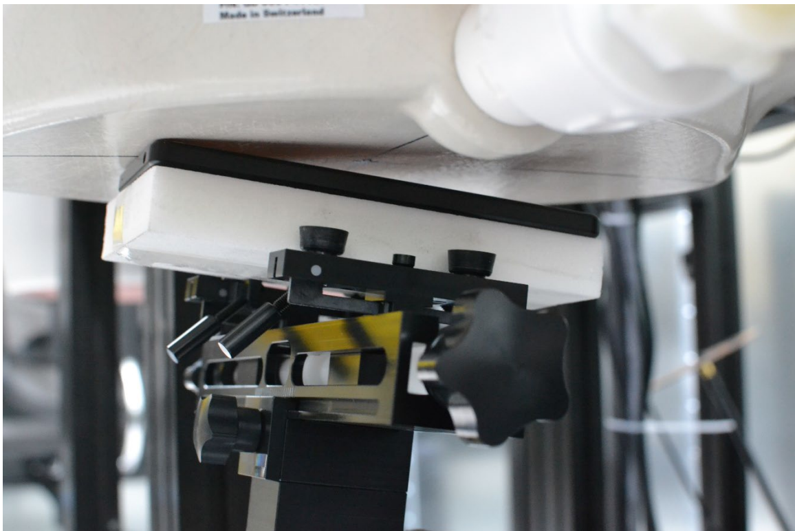
SAR Test Setup Photo 2 – Head, Right Cheek, Mouth Jaw for NR Band 41 at 0mm
