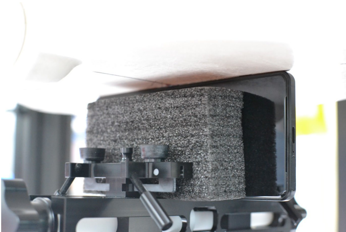
SAR Test Setup Photo 18 – Phablet, Right Side at 0mm
