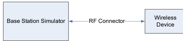
Figure 9-3 Power Measurement Setup
