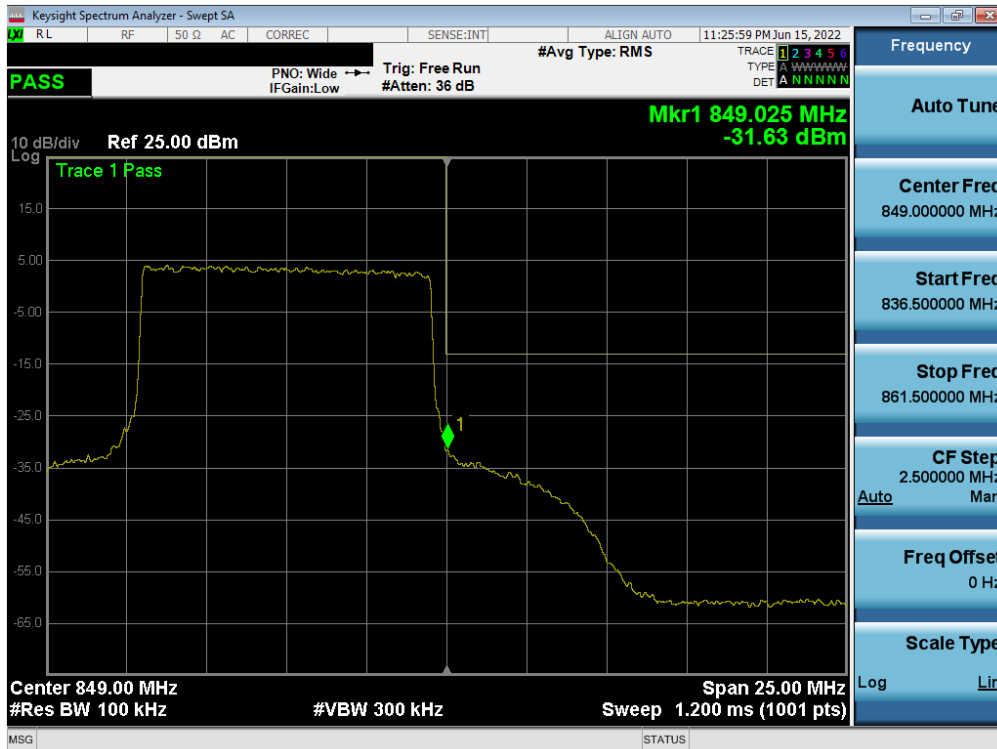
Plot 7-107. Upper Band Edge Plot (LTE Band 5 - 10MHz QPSK – Full RB – Sub ANT)
