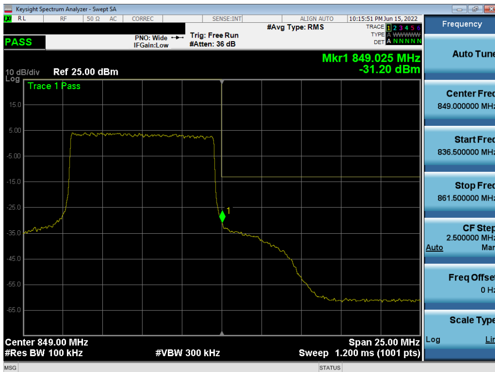
Plot 7-99. Upper Band Edge Plot (LTE Band 5 - 10MHz QPSK – Full RB – Main ANT)
