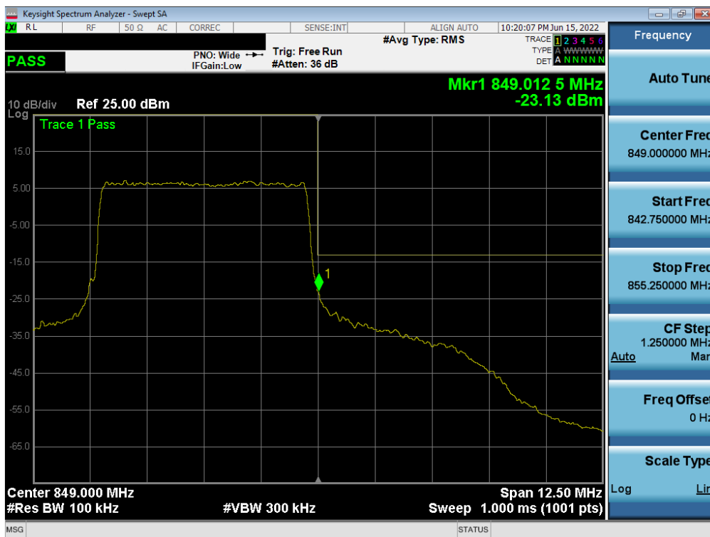
Plot 7-101. Upper Band Edge Plot (LTE Band 5 - 5MHz QPSK – Full RB – Main ANT)
