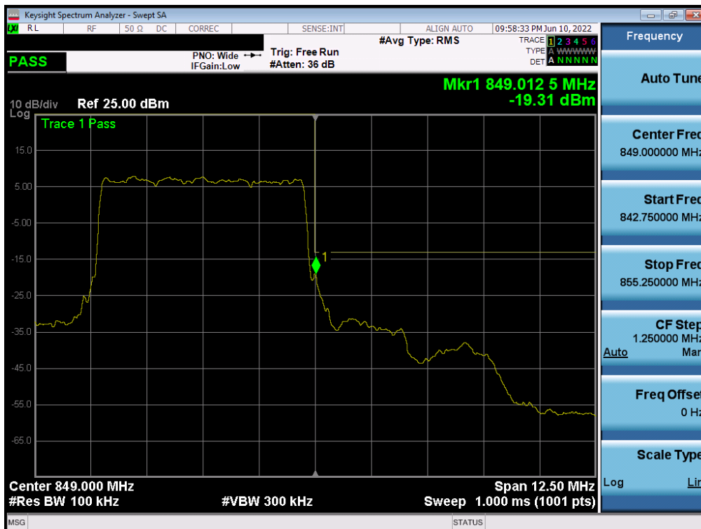
Plot 7-129. Upper Band Edge Plot (NR Band n5 - 5.0MHz - Full RB - Sub ANT)
