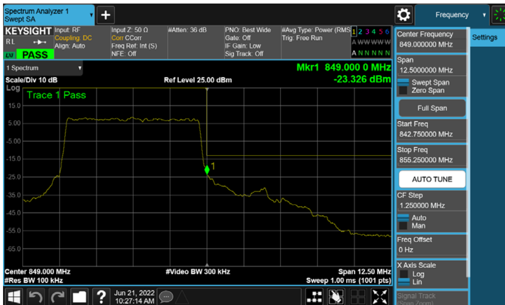
Plot 7-121. Upper Band Edge Plot (NR Band n5 – 5.0MHz - Full RB – Main ANT)
