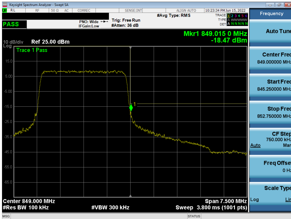
Plot 7-103. Upper Band Edge Plot (LTE Band 5 - 3MHz QPSK – Full RB – Main ANT)
