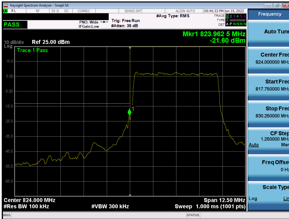
Plot 7-128. Lower Band Edge Plot (NR Band n5 - 5.0MHz - Full RB - Sub ANT)
