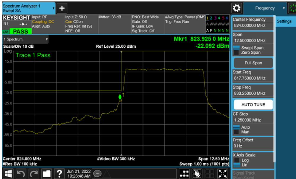
Plot 7-120. Lower Band Edge Plot (NR Band n5 – 5.0MHz - Full RB – Main ANT)
