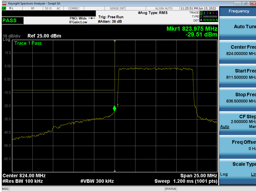
Plot 7-106. Lower Band Edge Plot (LTE Band 5 - 10MHz QPSK – Full RB – Sub ANT)
