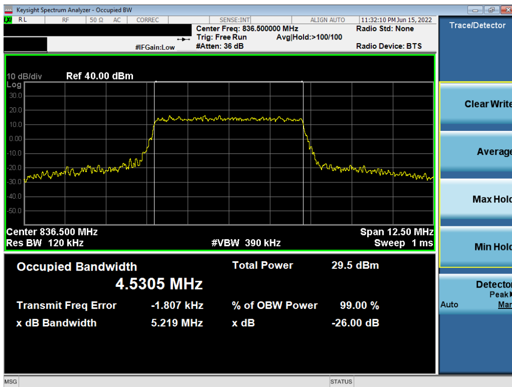
Plot 7-12. Occupied Bandwidth Plot (LTE Band 5 - 5MHz 16-QAM - Full RB – Sub ANT)
