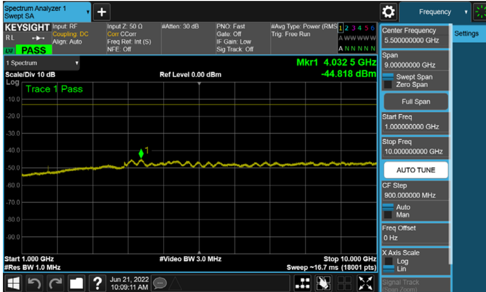
Plot 7-64. Conducted Spurious Plot (NR Band n5 - 20.0MHz - 1 RB - Low Channel – Main ANT)
