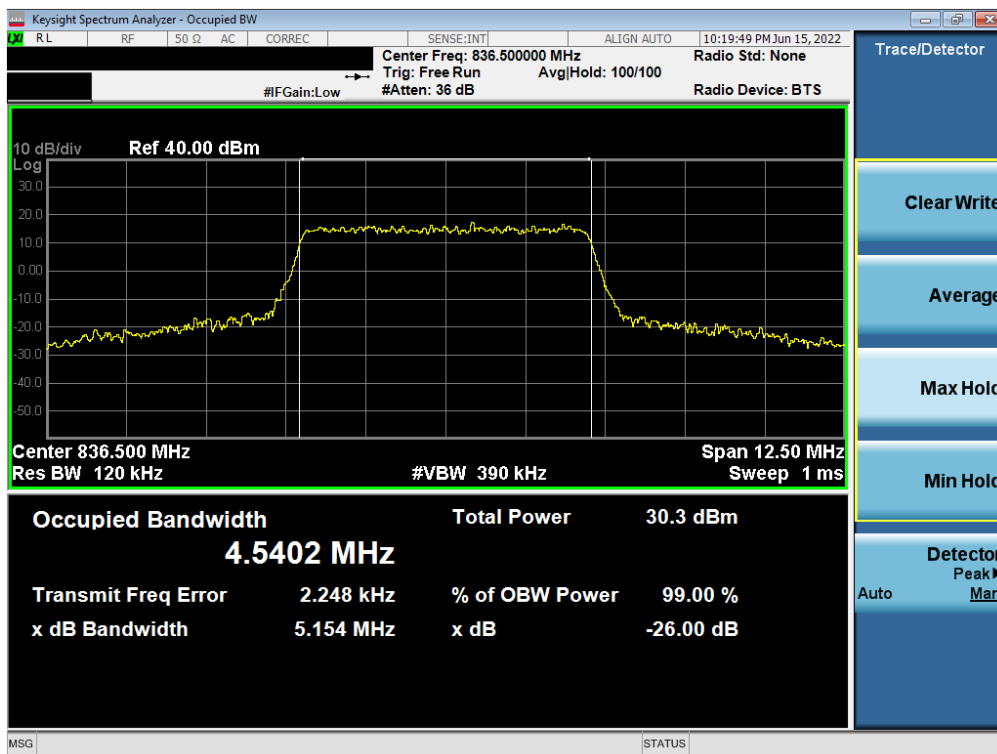
Plot 7-4. Occupied Bandwidth Plot (LTE Band 5 - 5MHz 16-QAM - Full RB - Main ANT)
