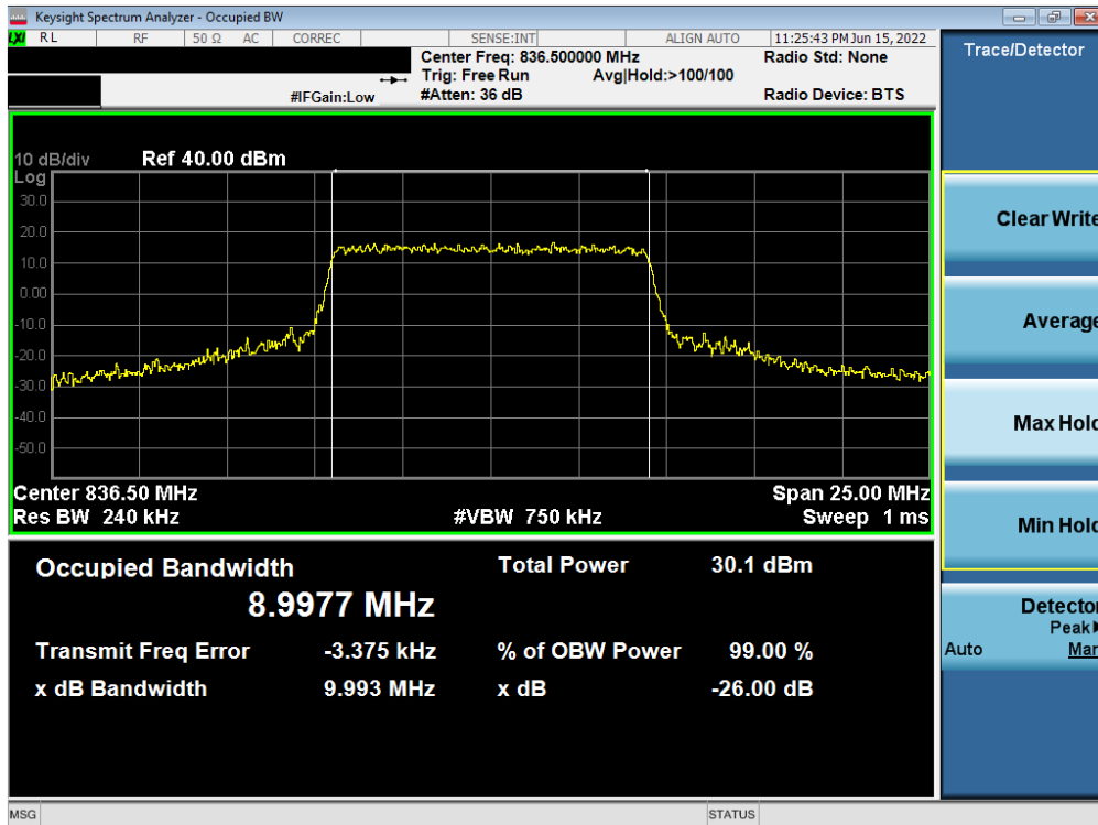
Plot 7-10. Occupied Bandwidth Plot (LTE Band 5 - 10MHz 16-QAM - Full RB – Sub ANT)
