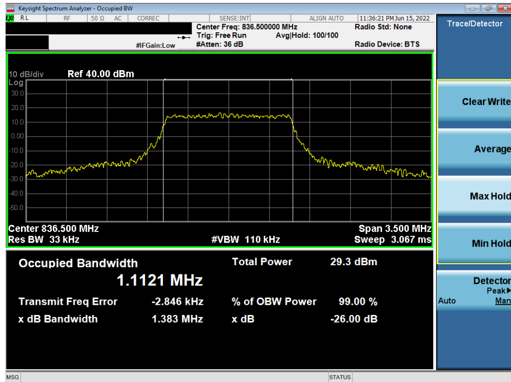
Plot 7-16. Occupied Bandwidth Plot (LTE Band 5 - 1.4MHz 16-QAM - Full RB – Sub ANT)
