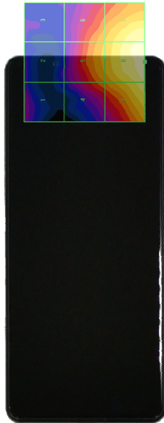
Figure 18-4 E-Field WD Scan overlay
