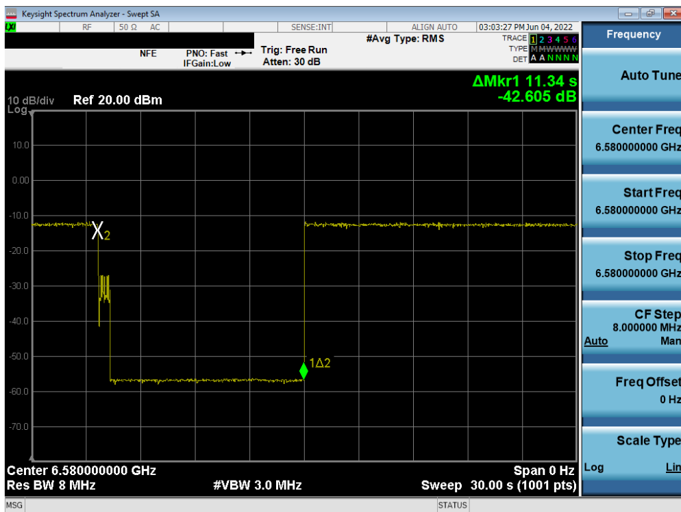
Plot 7-504. Contention Based Protocol Timing Plot – UNII 6 – 160MHz Ch111 - High
