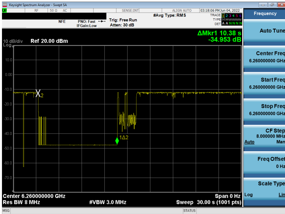
Plot 7-500. Contention Based Protocol Timing Plot – UNII 5 – 160MHz Ch47 - High
