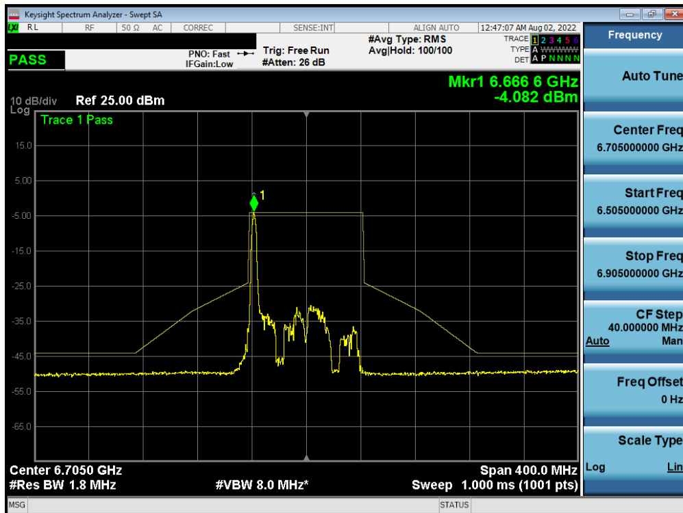
Plot 7-348. In-Band Emission Plot MIMO ANT1 (80MHz BW 802.11ax (26 Tones) (UNII Band 7) – Ch. 151)
