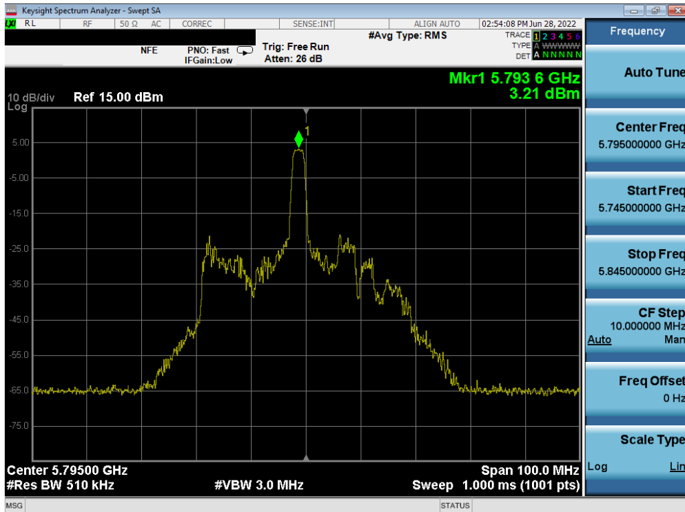
Plot 7-150. Power Spectral Density Plot MIMO ANT1 (40MHz BW 802.11ax – 26 Tones (UNII Band 3) – Ch. 159)
