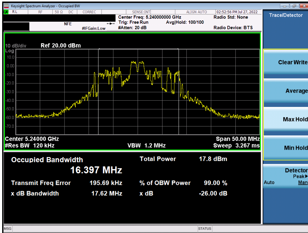
Plot 7-51. 26dB Bandwidth Plot MIMO ANT2 (20MHz BW 802.11ax – 26 Tones (UNII Band 1) – Ch. 48)
