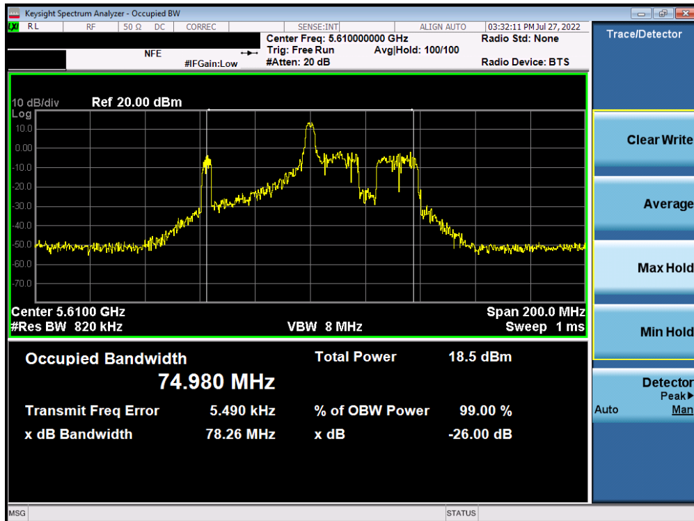
Plot 7-70. 26dB Bandwidth Plot MIMO ANT2 (80MHz BW 802.11ax – 26 Tones (UNII Band 2C) – Ch. 122)
