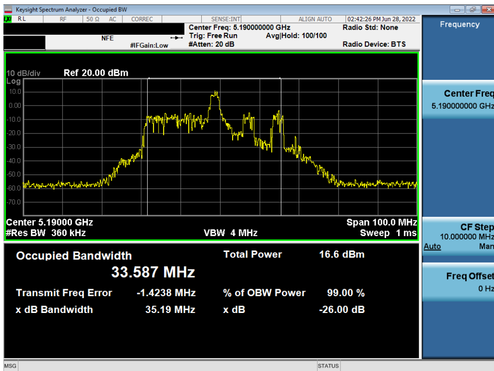
Plot 7-4. 26dB Bandwidth Plot MIMO ANT1 (40MHz BW 802.11ax – 26 Tones (UNII Band 1) – Ch. 38)
