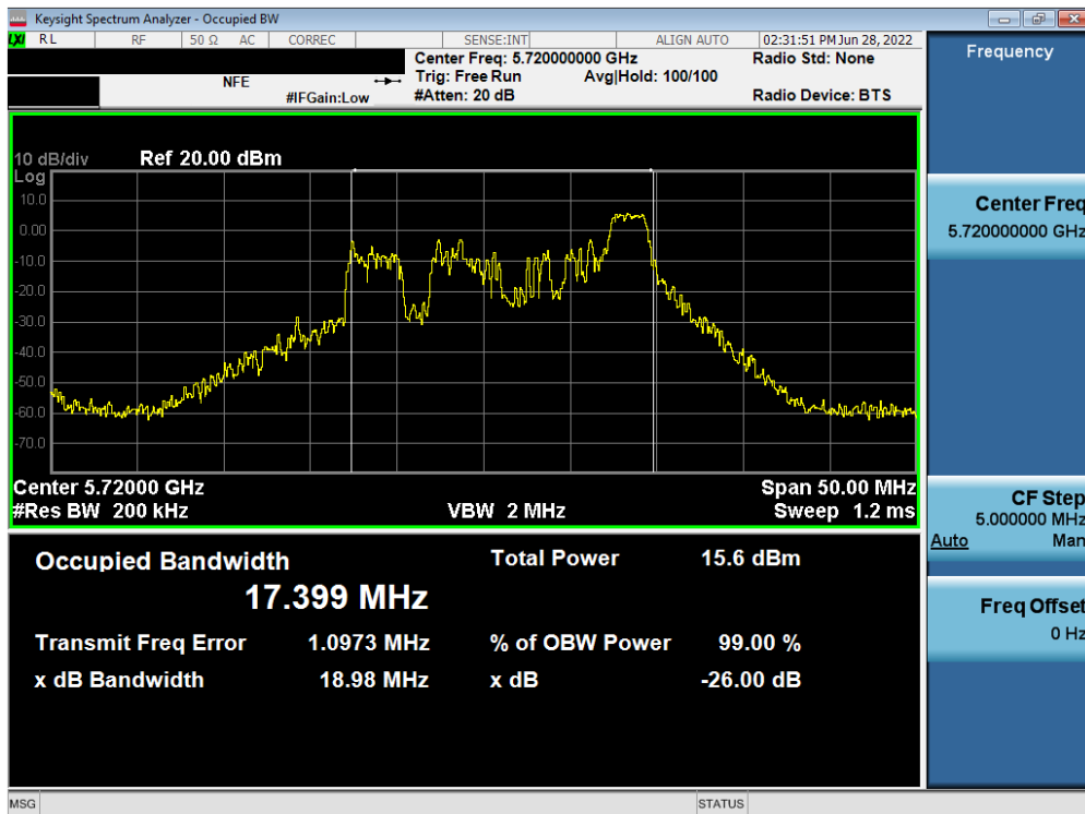
Plot 7-17. 26dB Bandwidth Plot MIMO ANT1 (20MHz BW 802.11ax – 26 Tones (UNII Band 2C) – Ch. 144)
