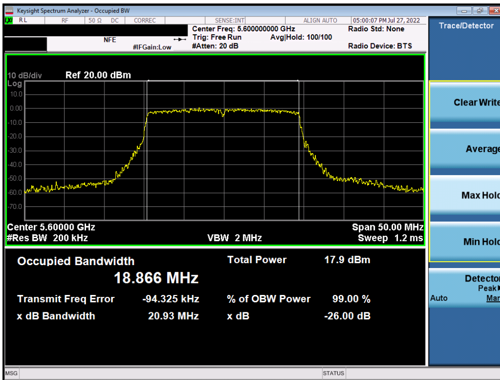
Plot 7-95. 26dB Bandwidth Plot MIMO ANT2 (802.11ax – 20MHz BW (UNII Band 2C) – Ch. 120)
