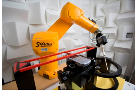
Figure 4-3 SPEAG Robotic System
