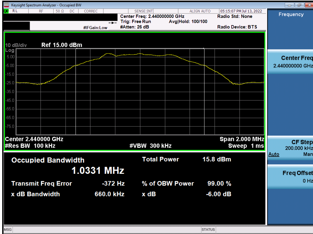
Plot 7-17. 6dB Bandwidth Plot (Bluetooth (LE), 500kbps – Ch. 19) – ANT 2
