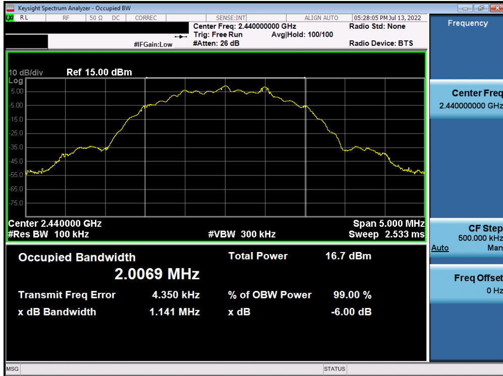
Plot 7-23. 6dB Bandwidth Plot (Bluetooth (LE), 2Mbps - Ch. 19) – ANT 2
