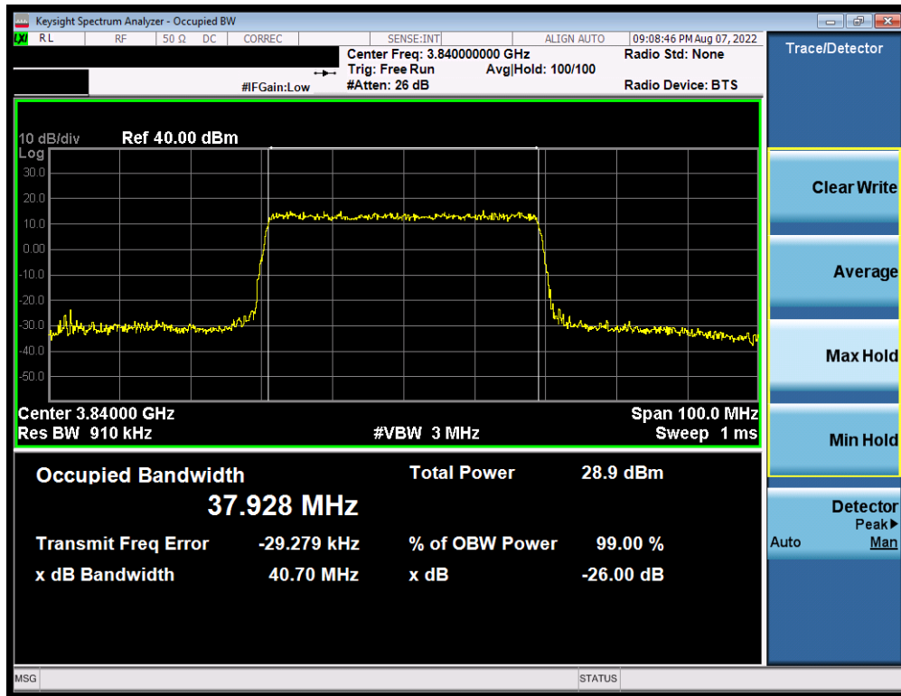
Plot 7-43. Occupied Bandwidth Plot (NR Band n77 - 40MHz QPSK - Full RB - Sub ANT (UL-MIMO))
