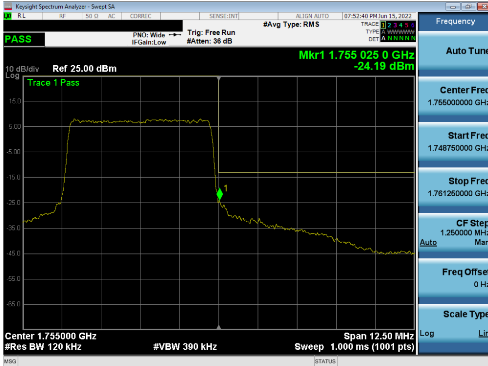
Plot 7-180. Upper Band Edge Plot (LTE Band 4 - 5MHz QPSK – Full RB Configuration)
