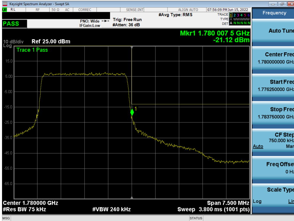
Plot 7-188. Upper Band Edge Plot (LTE Band 66 - 3MHz QPSK – Full RB Configuration)
