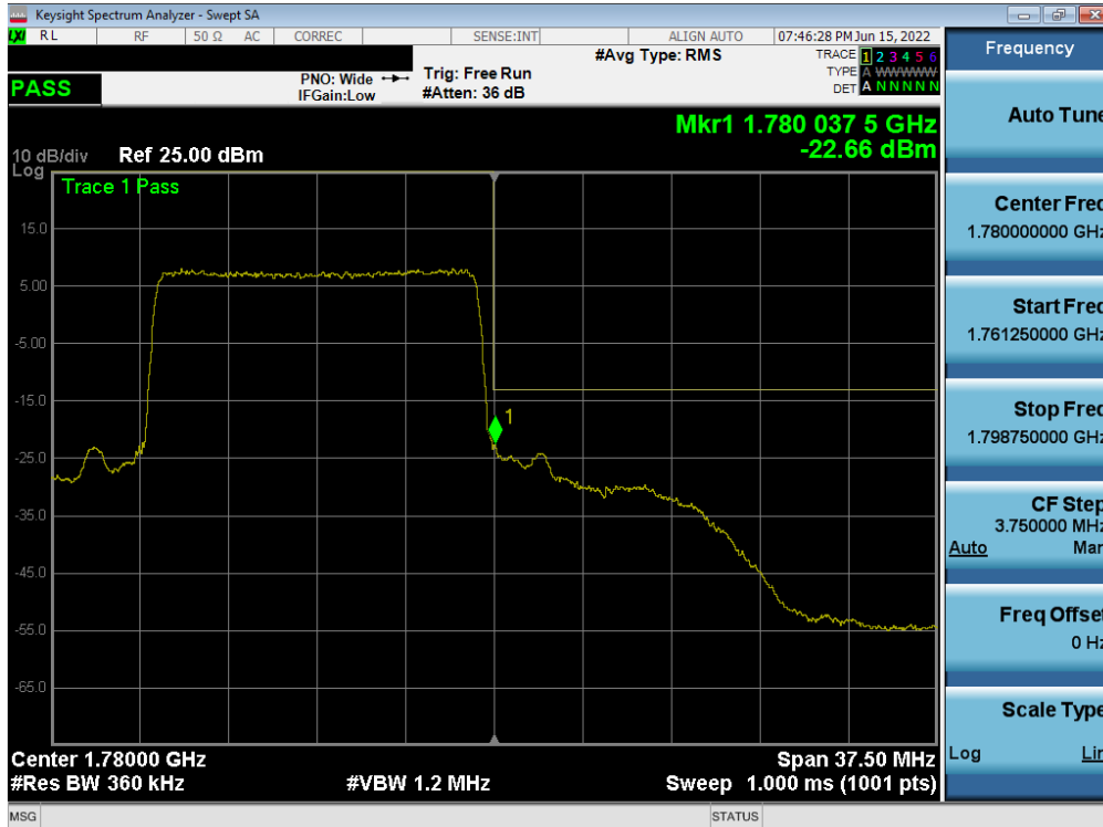
Plot 7-170. Upper Band Edge Plot (LTE Band 66 - 15MHz QPSK – Full RB Configuration)
