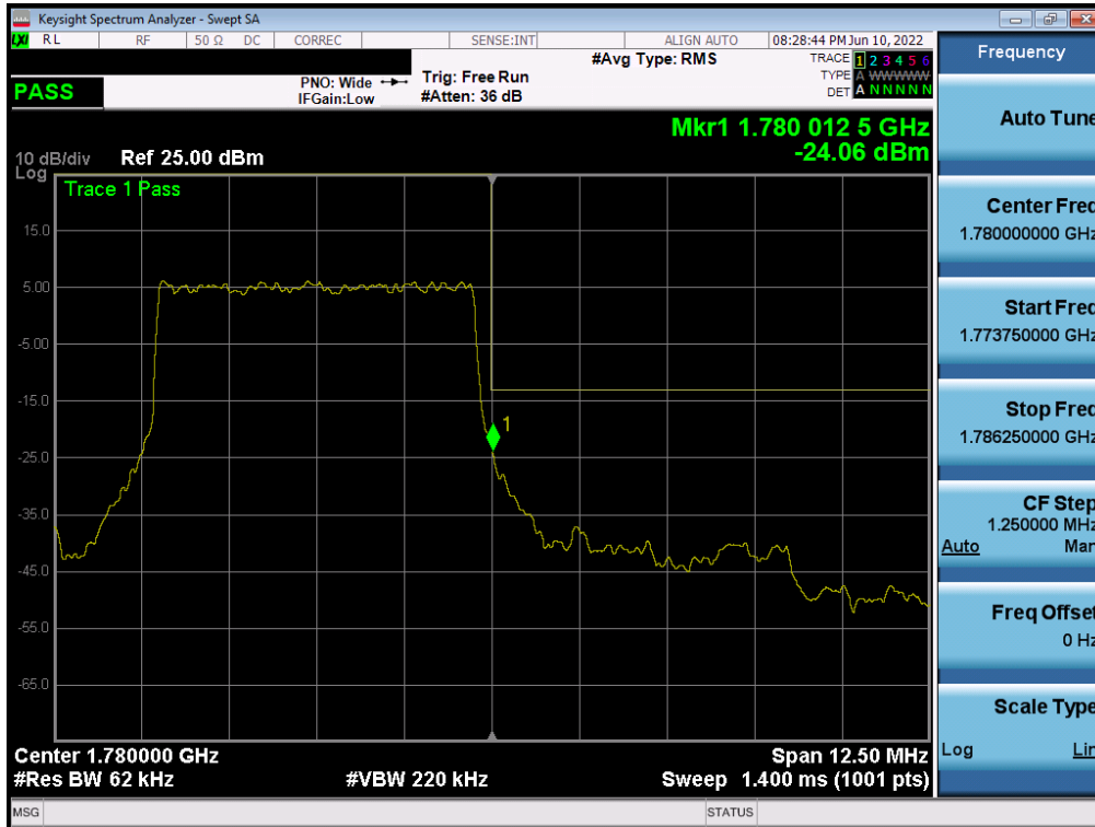
Plot 7-210. Upper Band Edge Plot (NR Band n66 – 5.0MHz - Full RB)
