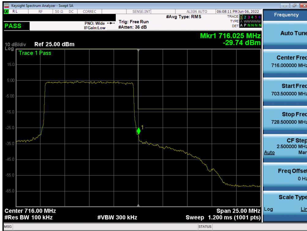
Plot 7-140. Upper Band Edge Plot (LTE Band 12/17 - 10MHz QPSK – Full RB Configuration – Main ANT)
