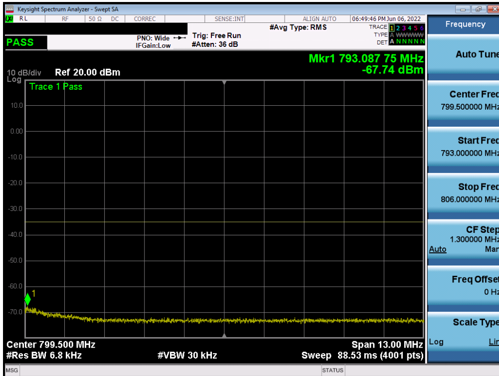
Plot 7-155. Upper Emission Mask Plot (LTE Band 13 - 5MHz QPSK – Full RB Configuration – Main ANT)
