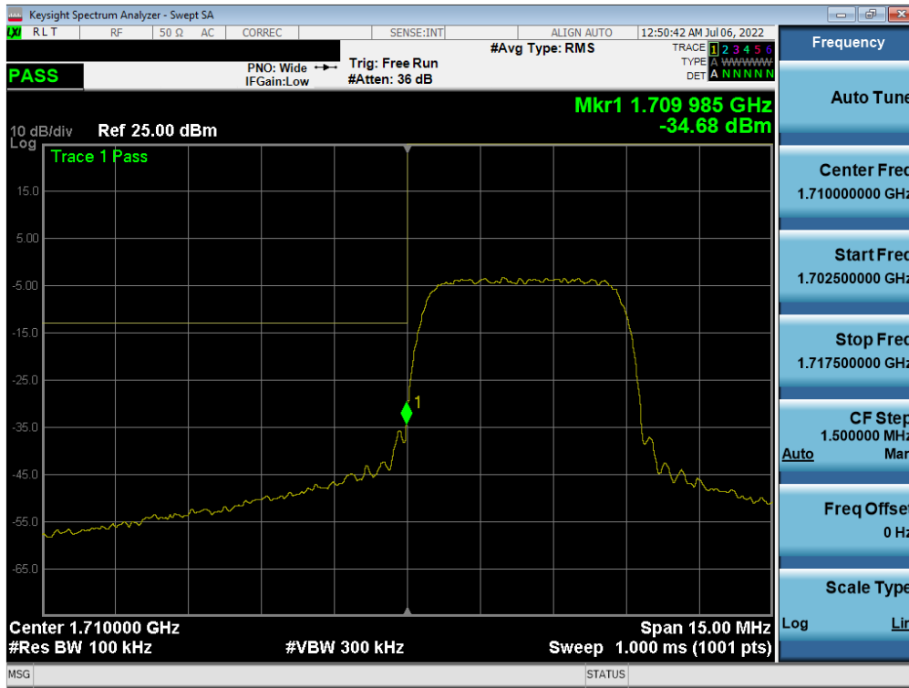
Plot 7-156. Lower Band Edge Plot (WCDMA AWS – Ch. 1312)
