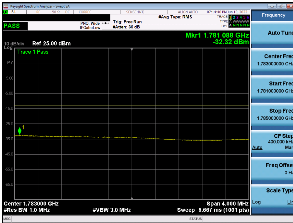
Plot 7-199. Upper Extended Band Edge Plot (NR Band n66 – 20.0MHz - Full RB)
