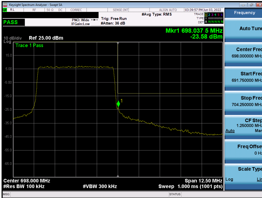
Plot 7-137. Upper Band Edge Plot (LTE Band 71 - 5MHz QPSK – Full RB Configuration)
