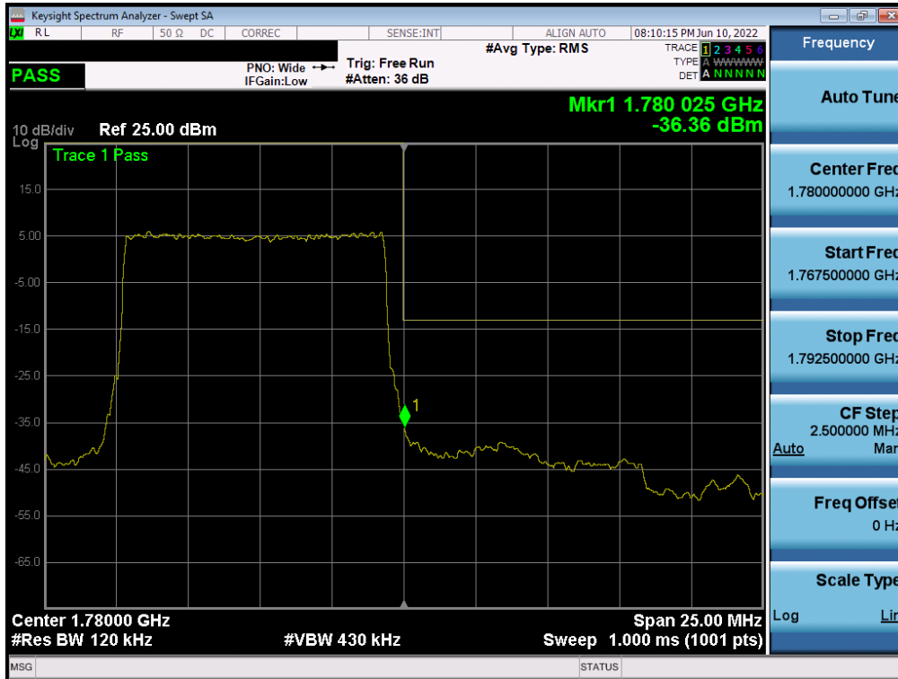
Plot 7-206. Upper Band Edge Plot (NR Band n66 - 10.0MHz - Full RB)
