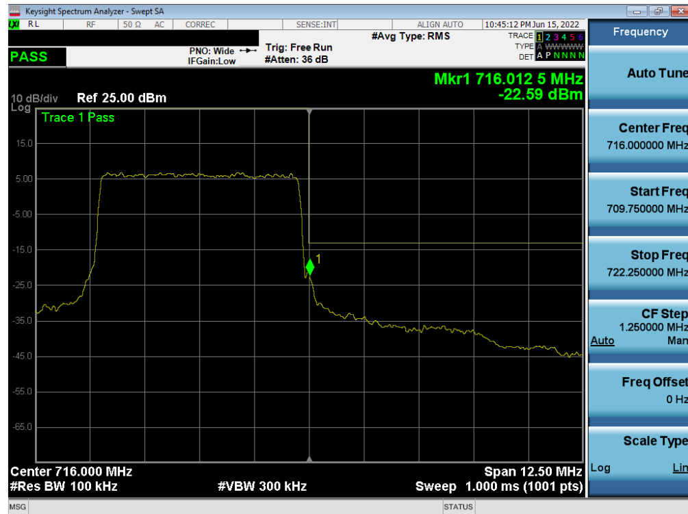
Plot 7-217. Upper Band Edge Plot (LTE Band 12/17 - 5MHz QPSK – Full RB Configuration – Sub ANT)
