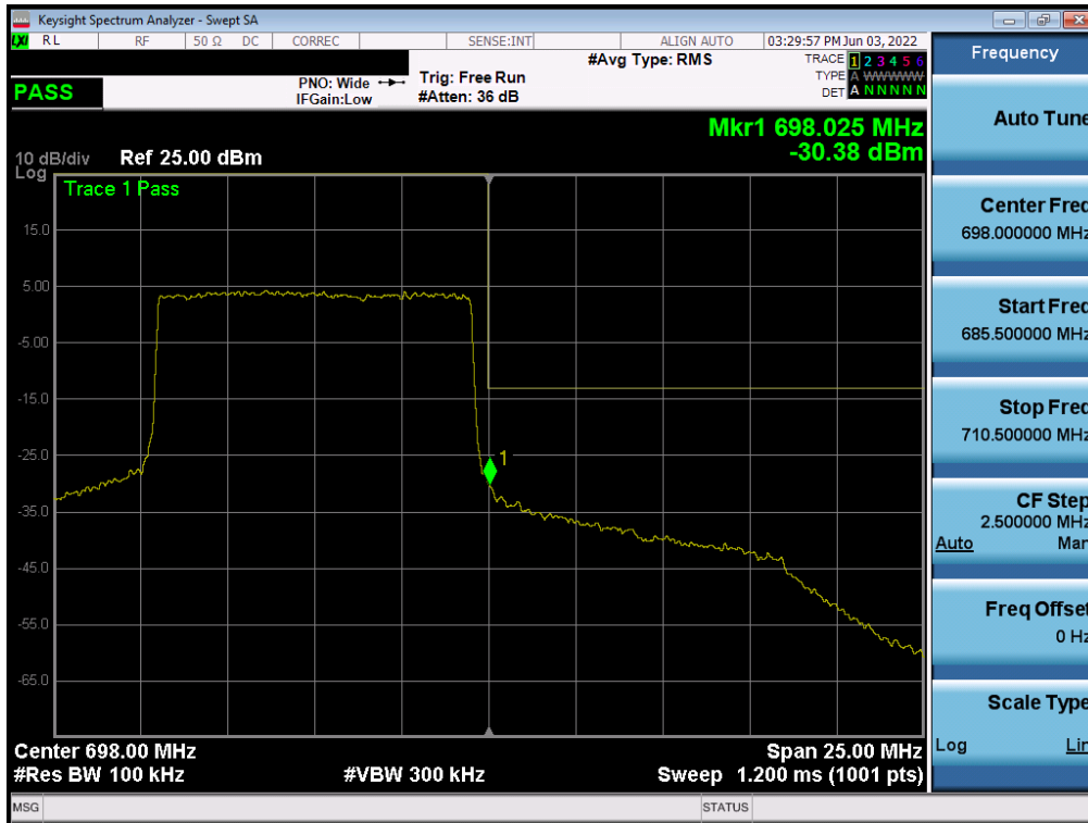
Plot 7-135. Upper Band Edge Plot (LTE Band 71 - 10MHz QPSK – Full RB Configuration)
