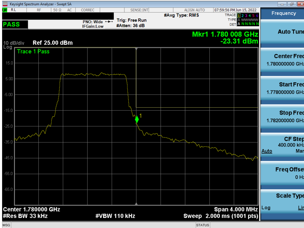
Plot 7-194. Upper Band Edge Plot (LTE Band 66 – 1.4MHz QPSK – Full RB Configuration)
