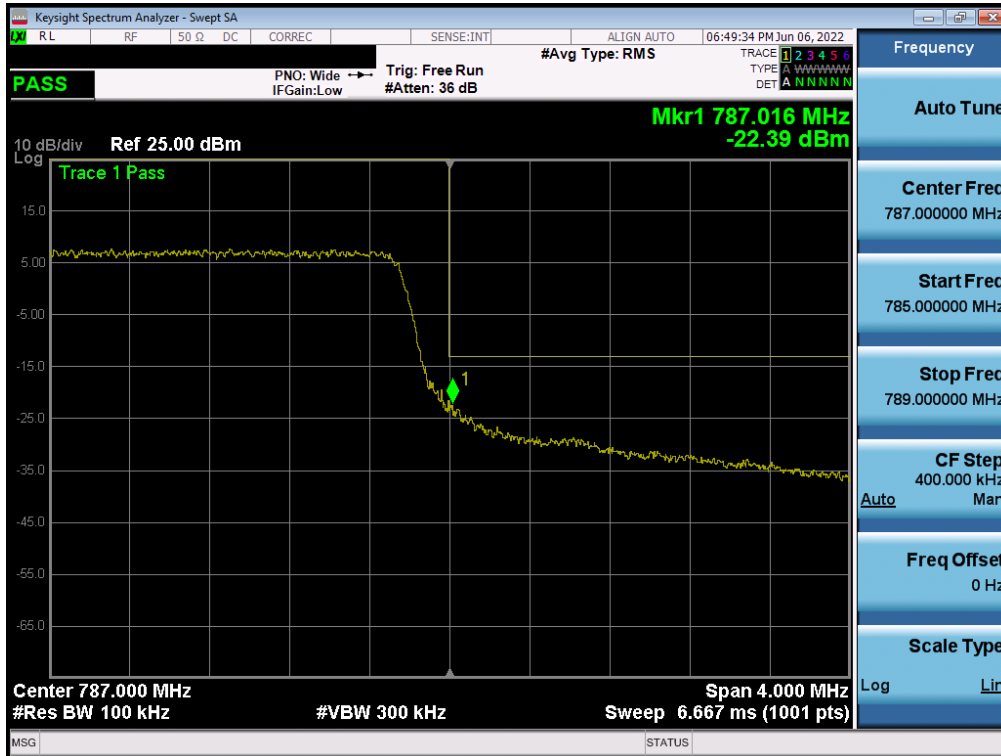
Plot 7-154. Upper Band Edge Plot (LTE Band 13 - 5MHz QPSK – Full RB Configuration – Main ANT)
