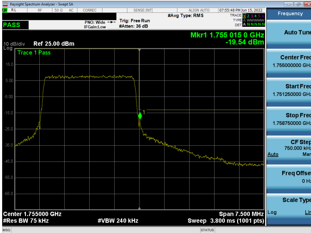
Plot 7-186. Upper Band Edge Plot (LTE Band 4 - 3MHz QPSK – Full RB Configuration)
