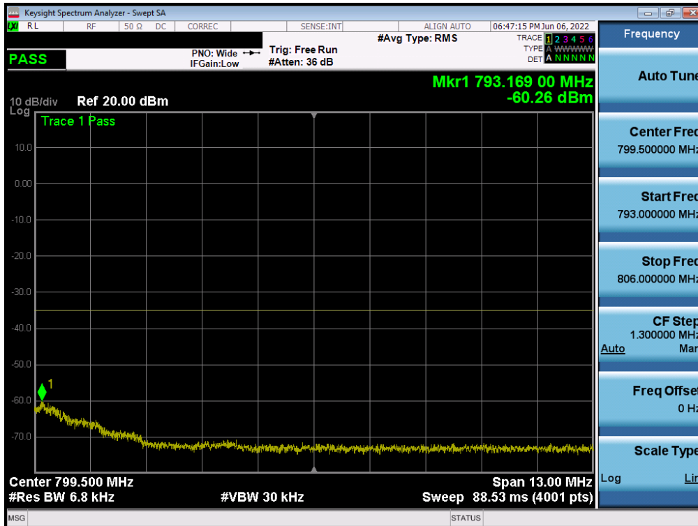
Plot 7-151. Upper Emission Mask Plot (LTE Band 13 - 10MHz QPSK – Full RB Configuration – Main ANT)
