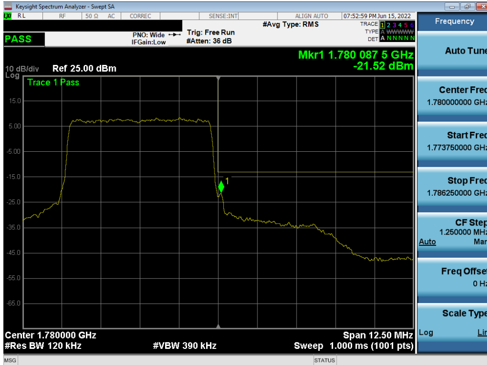
Plot 7-182. Upper Band Edge Plot (LTE Band 66 - 5MHz QPSK – Full RB Configuration)
