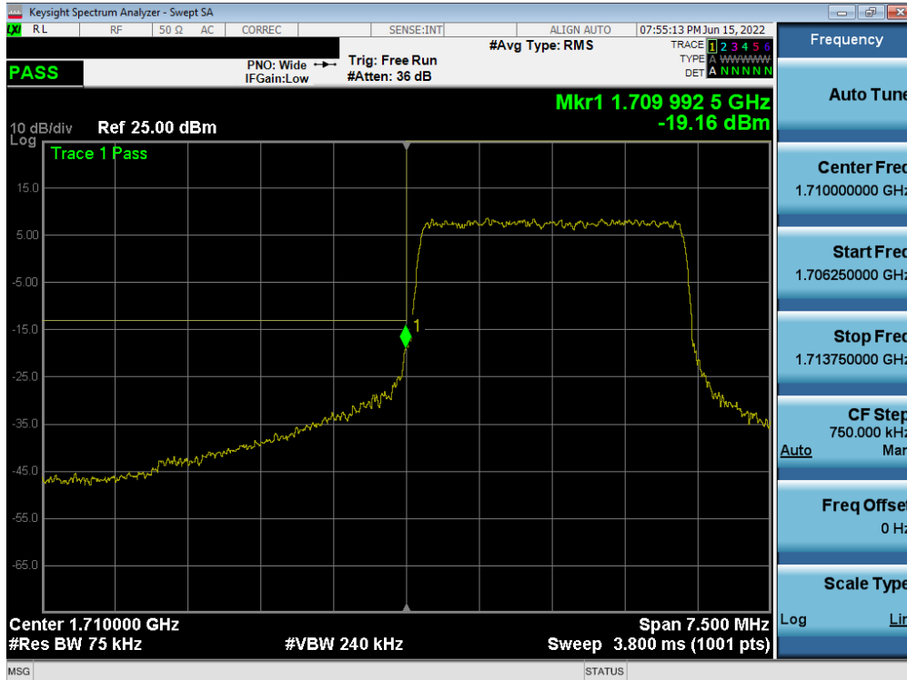
Plot 7-184. Lower Band Edge Plot (LTE Band 66/4 - 3MHz QPSK – Full RB Configuration)
