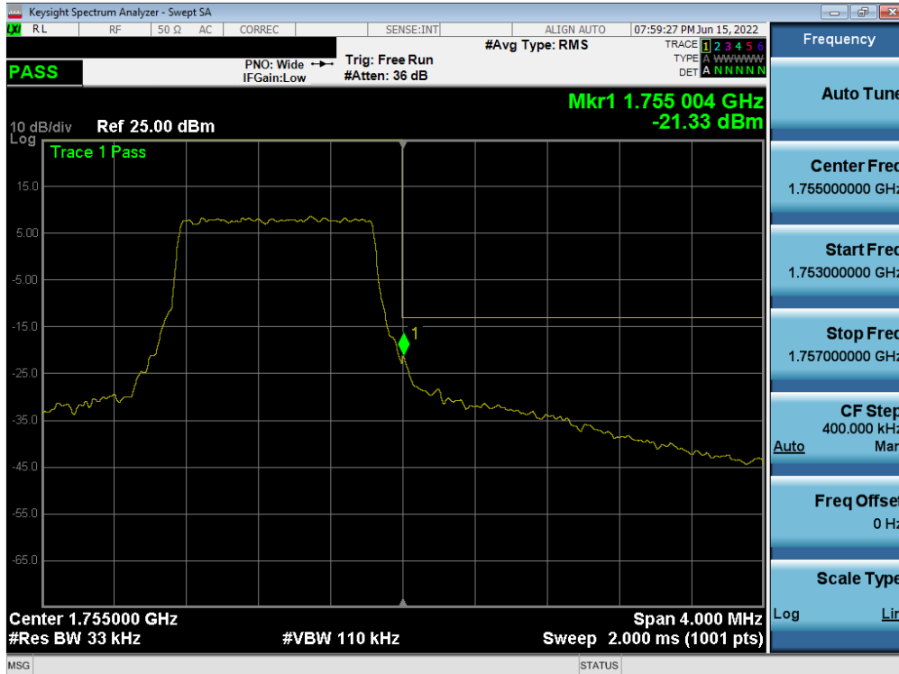
Plot 7-192. Upper Band Edge Plot (LTE Band 4 – 1.4MHz QPSK – Full RB Configuration)
