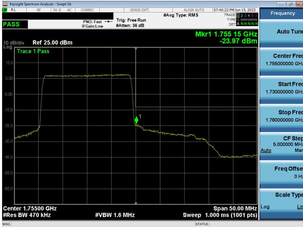
Plot 7-162. Upper Band Edge Plot (LTE Band 4 - 20MHz QPSK – Full RB Configuration)
