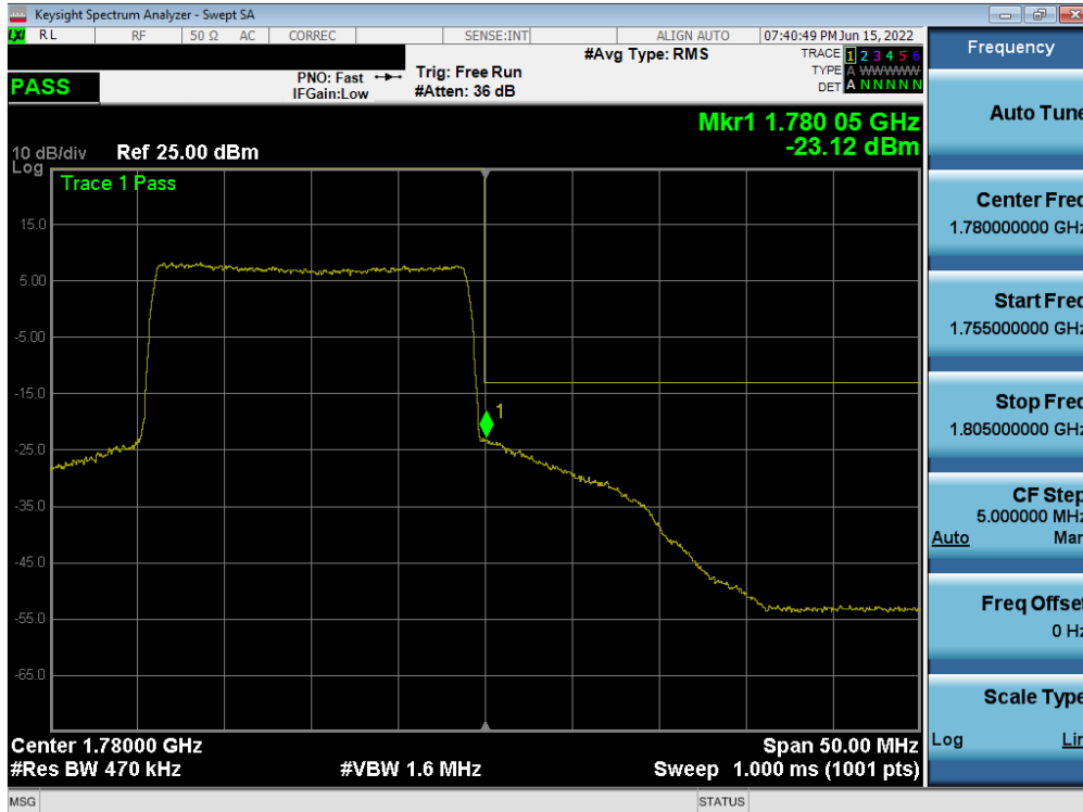
Plot 7-164. Upper Band Edge Plot (LTE Band 66 - 20MHz QPSK – Full RB Configuration)
