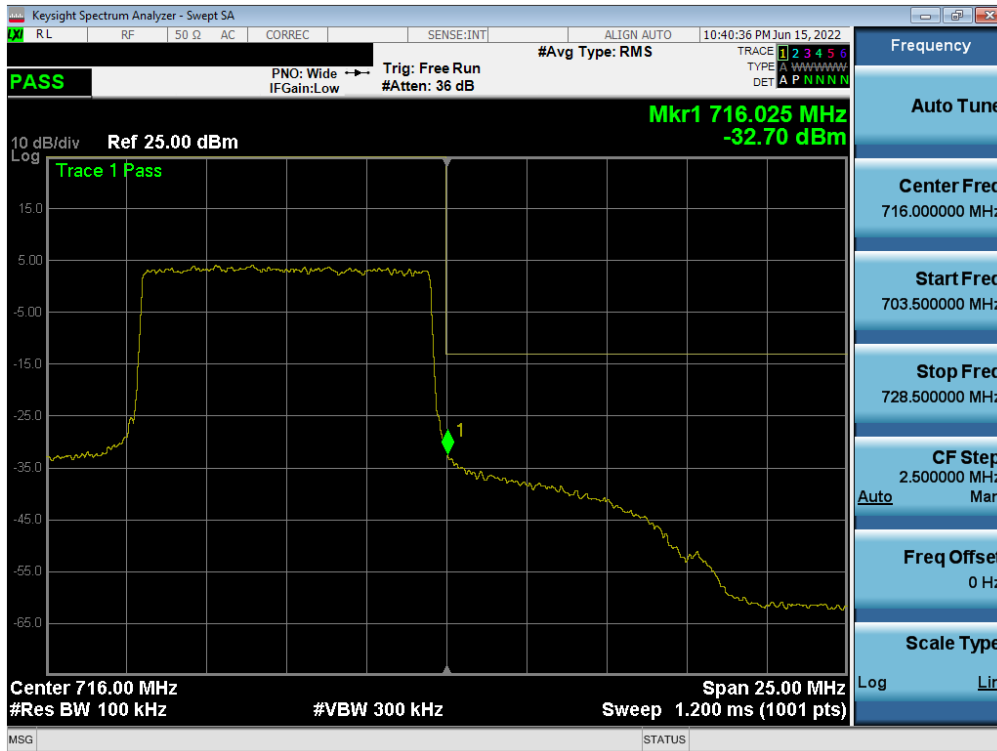
Plot 7-214. Upper Band Edge Plot (LTE Band 12/17 - 10MHz QPSK – Full RB Configuration – Sub ANT)
