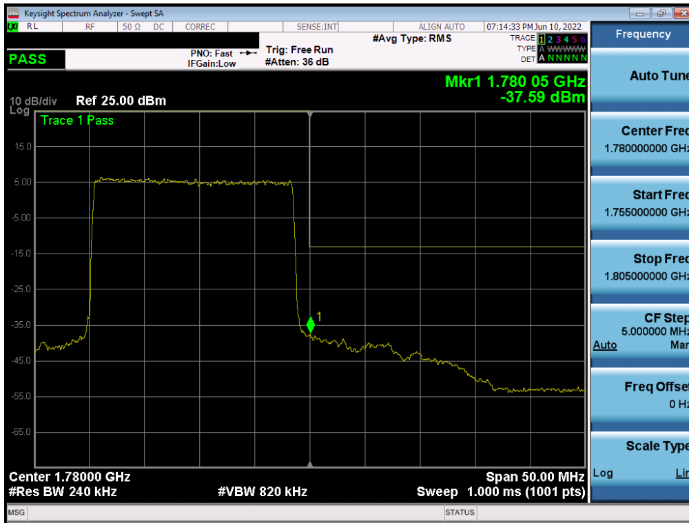
Plot 7-198. Upper Band Edge Plot (NR Band n66 – 20.0MHz - Full RB)
