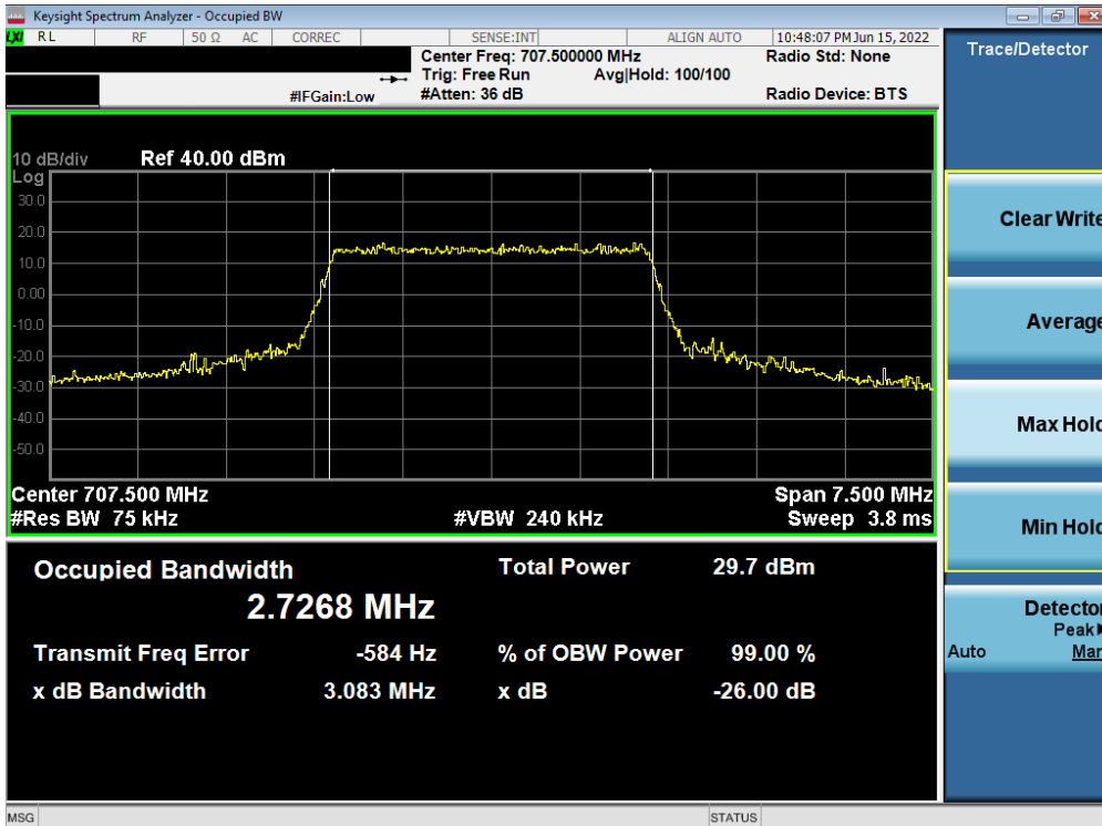
Plot 7-63. Occupied Bandwidth Plot (LTE Band 12/17 - 3MHz 16-QAM - Full RB Configuration – Sub ANT)
