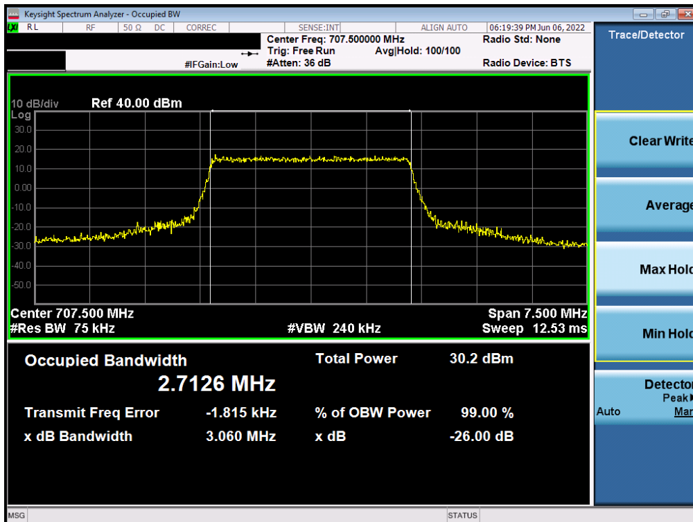
Plot 7-14. Occupied Bandwidth Plot (LTE Band 12/17 - 3MHz 16-QAM - Full RB Configuration – Main ANT)
