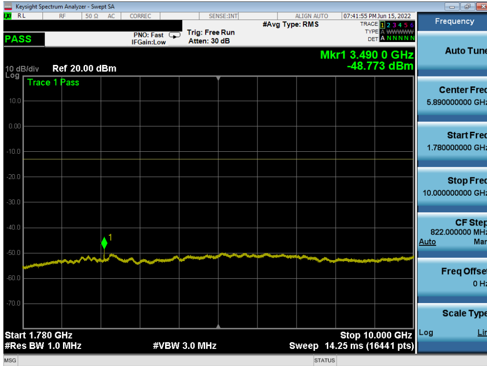
Plot 7-104. Conducted Spurious Plot (LTE Band 66/4 - 20MHz QPSK - 1 RB - Mid Channel)
