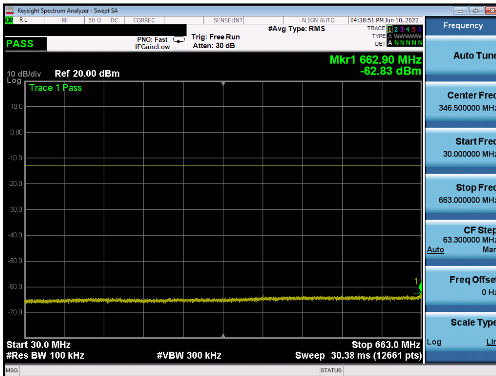
Plot 7-94. Conducted Spurious Plot (NR Band n71 - 20.0MHz - 1 RB - Mid Channel)
