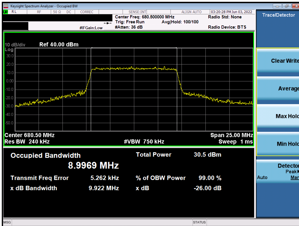
Plot 7-6. Occupied Bandwidth Plot (LTE Band 71 - 10MHz 16-QAM - Full RB Configuration)
