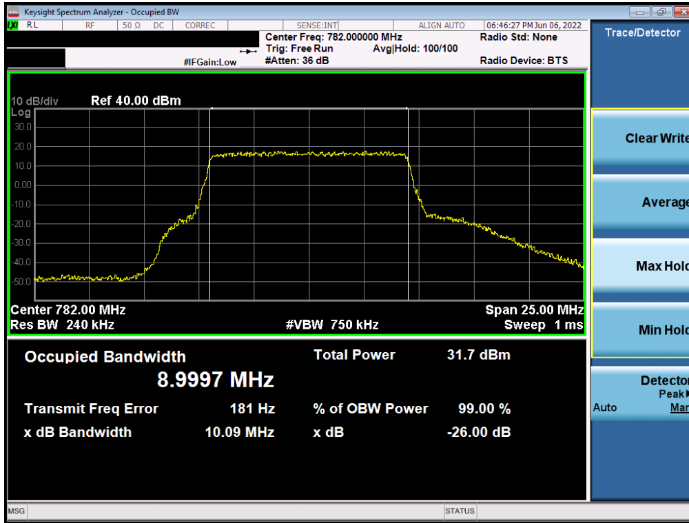
Plot 7-17. Occupied Bandwidth Plot (LTE Band 13 - 10MHz QPSK - Full RB Configuration – Main ANT)
