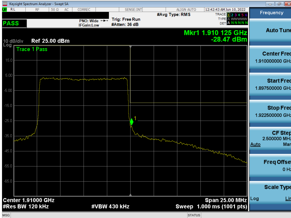
Plot 7-116. Upper Band Edge Plot (NR Band n2 – 10.0MHz - Full RB)
