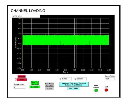
The level of traffic loading on the channel by the EUT is 69.572%.
