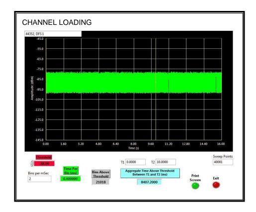
The level of traffic loading on the channel by the EUT is 84.072%.
