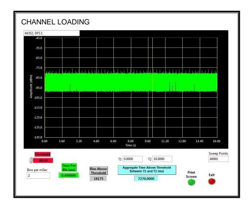
The level of traffic loading on the channel by the EUT is 72.7%.
