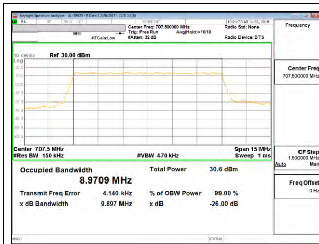
LTE B12 10MHz QPSK Mid Channel RB50-0
