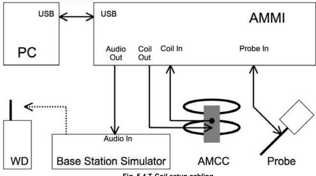
Fig. 5.4 T-Coil setup cabling
