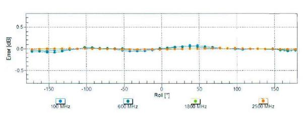
Receiving Pattern ( $\phi$ ),  $\vartheta = 0^{\circ}$
