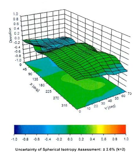
Deviation from Isotropy in Air Error (\oplus, \oplus), f = 900 MHz
