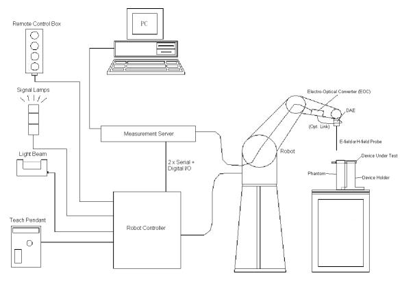
Fig 5.1 SPEAG DASY5 System Configurations
