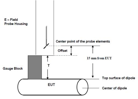
Fig. 8.3 Gauge block with E-field probe
