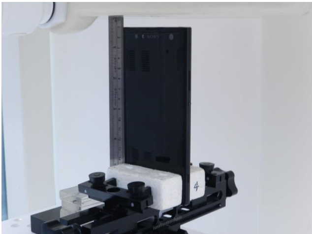
Top Side, Test Separation 10 mm
