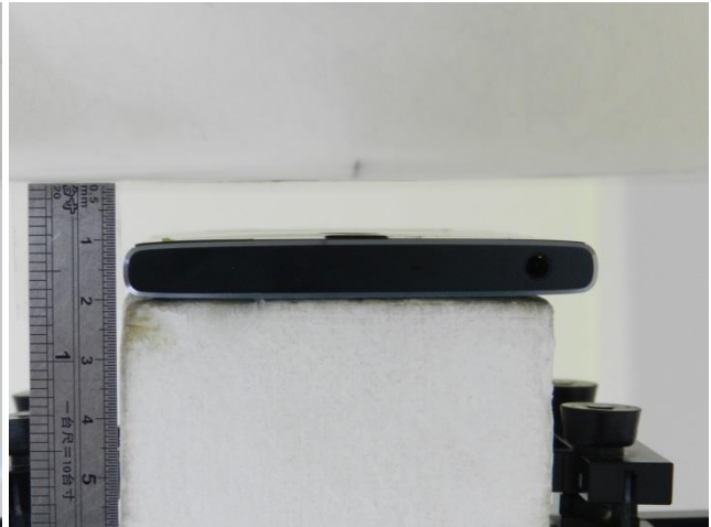
Back, Test Separation 10 mm
