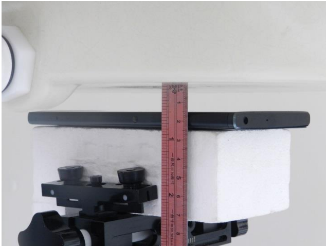
Front, Test Separation 15 mm
