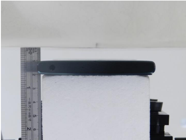
Front, Test Separation 10 mm
