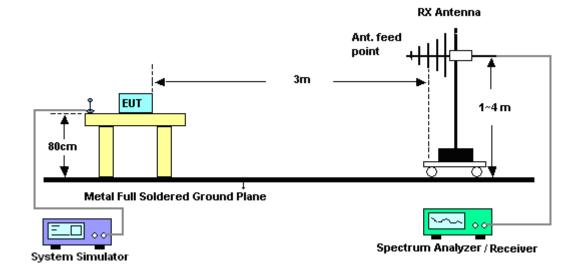
For radiated test above 1GHz
