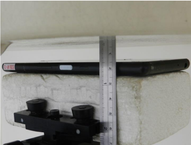
Front, Test Separation 15 mm
