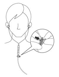
• Attach the clip to the headset cable below the remote. Position the clip so that you can speak into the microphone for taking calls hands-free, once the headset is fastened to your clothes.
