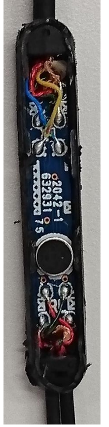
Controller box (Rear)
