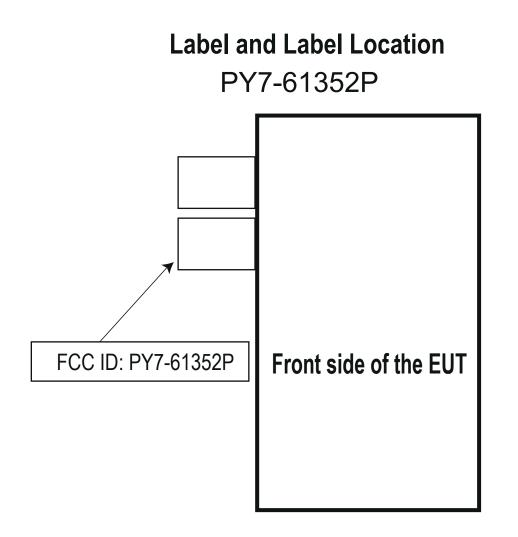
The FCC ID is not on the exterior of the device but labelling meets the conditions allowed in KDB 784748 for the label to be placed in a user accessible area:
