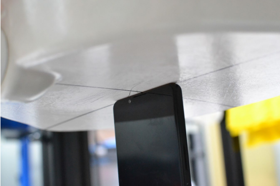
SAR Test Setup Photo 13 – Phablet, Top Side at 0mm
