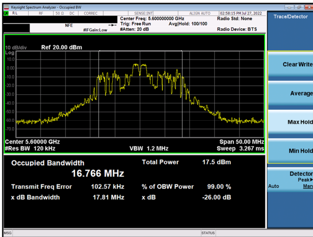
Plot 7-64. 26dB Bandwidth Plot MIMO ANT2 (20MHz BW 802.11ax – 26 Tones (UNII Band 2C) – Ch. 120)
