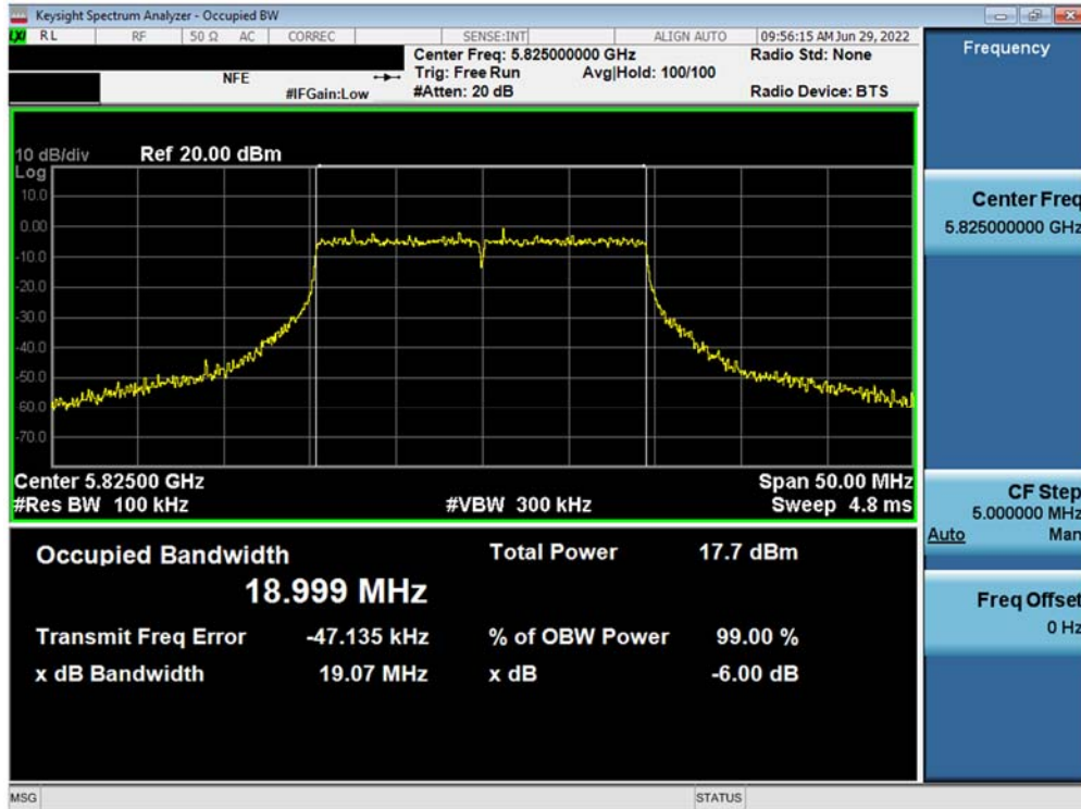
Plot 7-105. 6dB Bandwidth Plot MIMO ANT1 (20MHz BW 802.11ax – 242 Tones (UNII Band 3) – Ch. 165)
