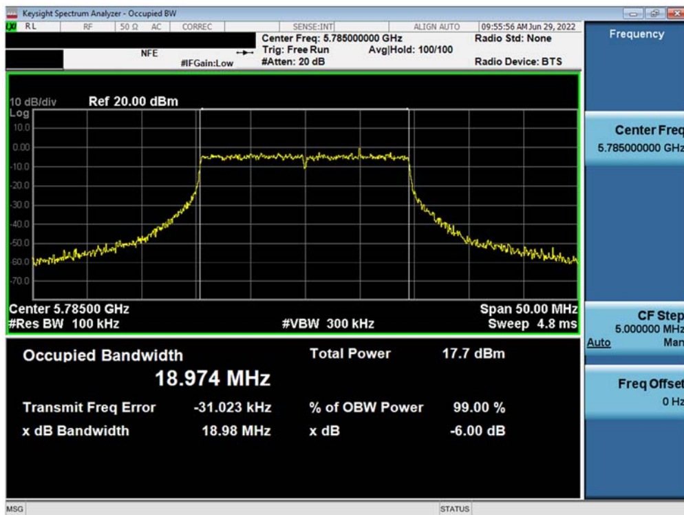
Plot 7-104. 6dB Bandwidth Plot MIMO ANT1 (20MHz BW 802.11ax – 242 Tones (UNII Band 3) – Ch. 157)
