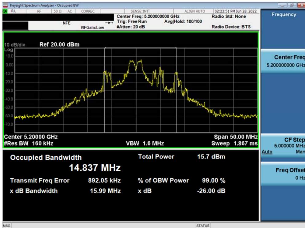
Plot 7-2. 26dB Bandwidth Plot MIMO ANT1 (20MHz BW 802.11ax – 26 Tones (UNII Band 1) – Ch. 40)
