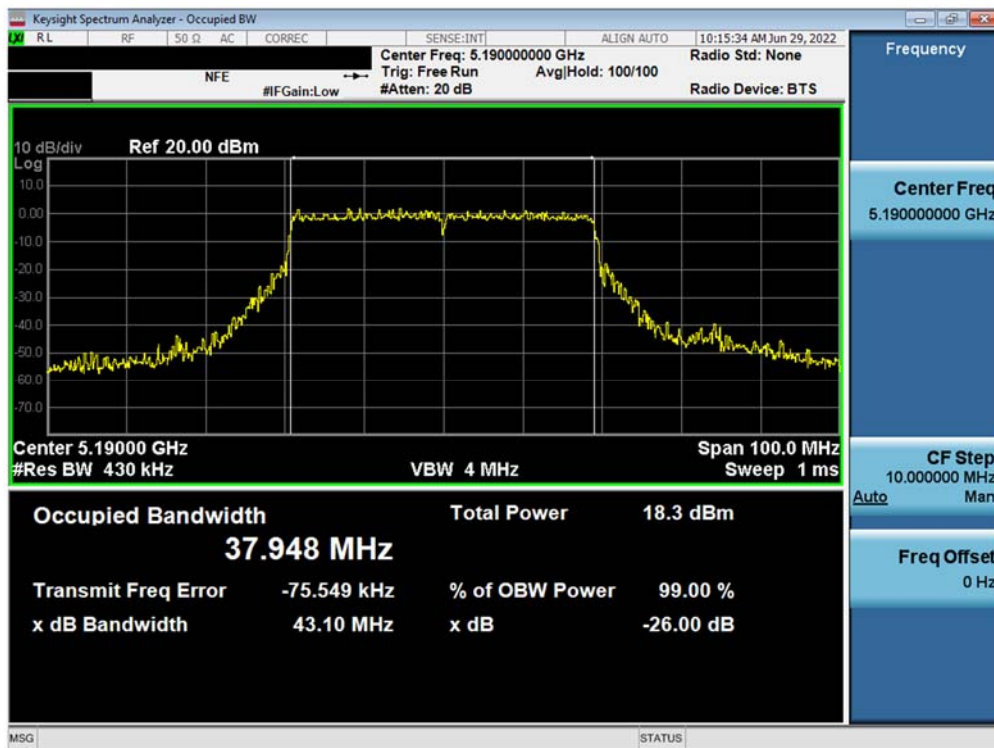
Plot 7-29. 26dB Bandwidth Plot MIMO ANT1 (40MHz BW 802.11ax – 484 Tones (UNII Band 1) – Ch. 38)
