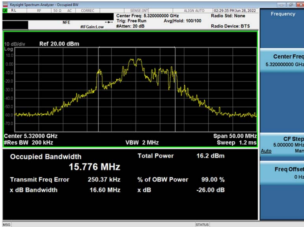
Plot 7-11. 26dB Bandwidth Plot MIMO ANT1 (20MHz BW 802.11ax – 26 Tones (UNII Band 2A) – Ch. 64)
