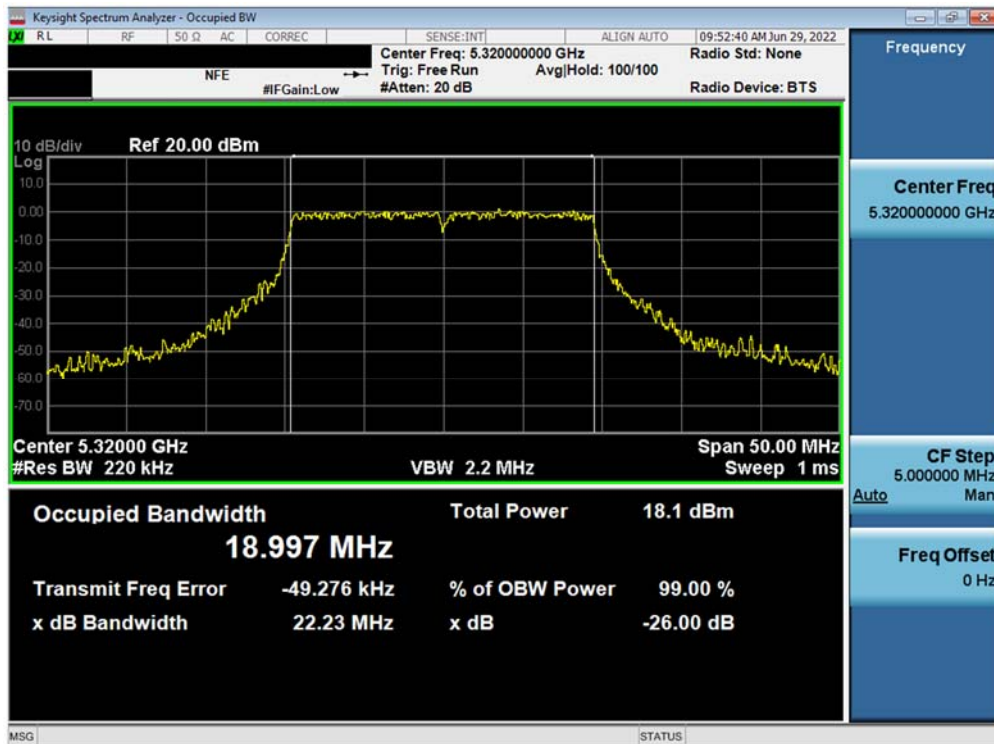
Plot 7-35. 26dB Bandwidth Plot MIMO ANT1 (20MHz BW 802.11ax – 242 Tones (UNII Band 2A) – Ch. 64)
