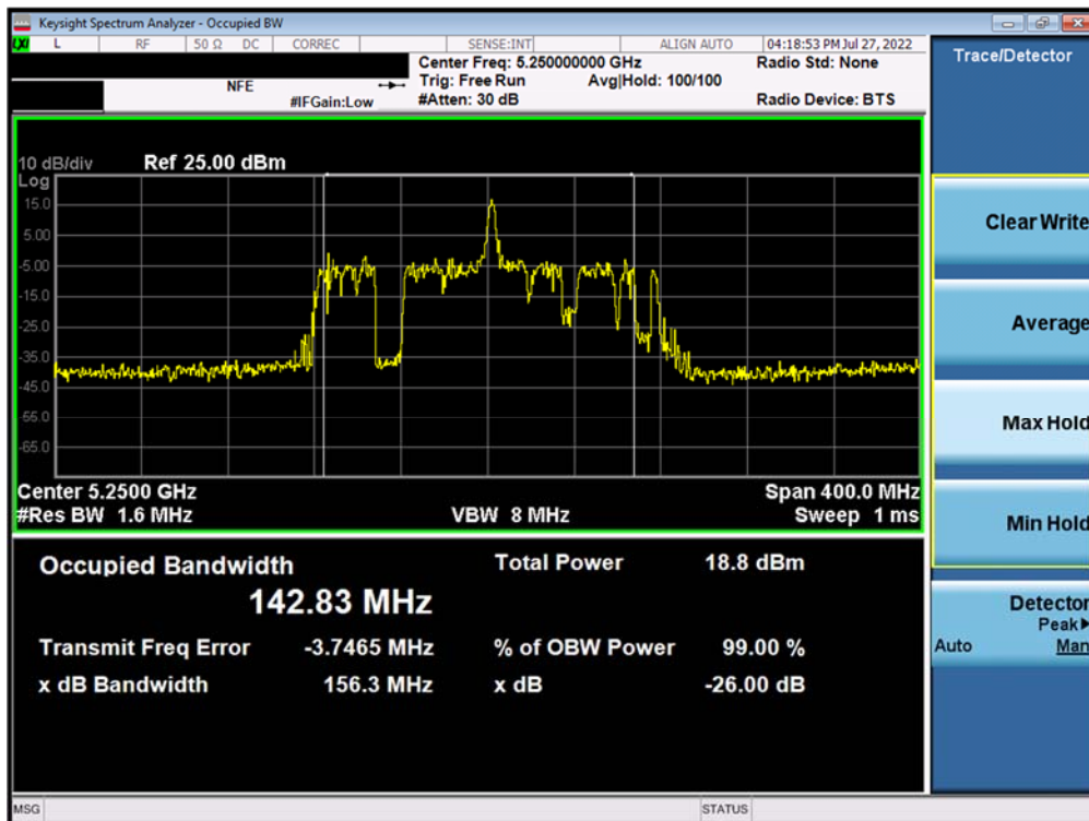
Plot 7-8. 26dB Bandwidth Plot MIMO ANT1 (160MHz U BW 802.11ax – 26 Tones (UNII Band 1/2A) – Ch. 50)
