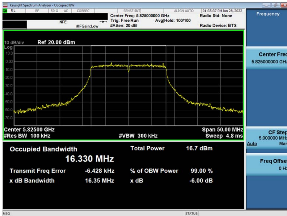
Plot 7-128. 6dB Bandwidth Plot MIMO ANT2 (802.11a (UNII Band 3) – Ch. 165)
