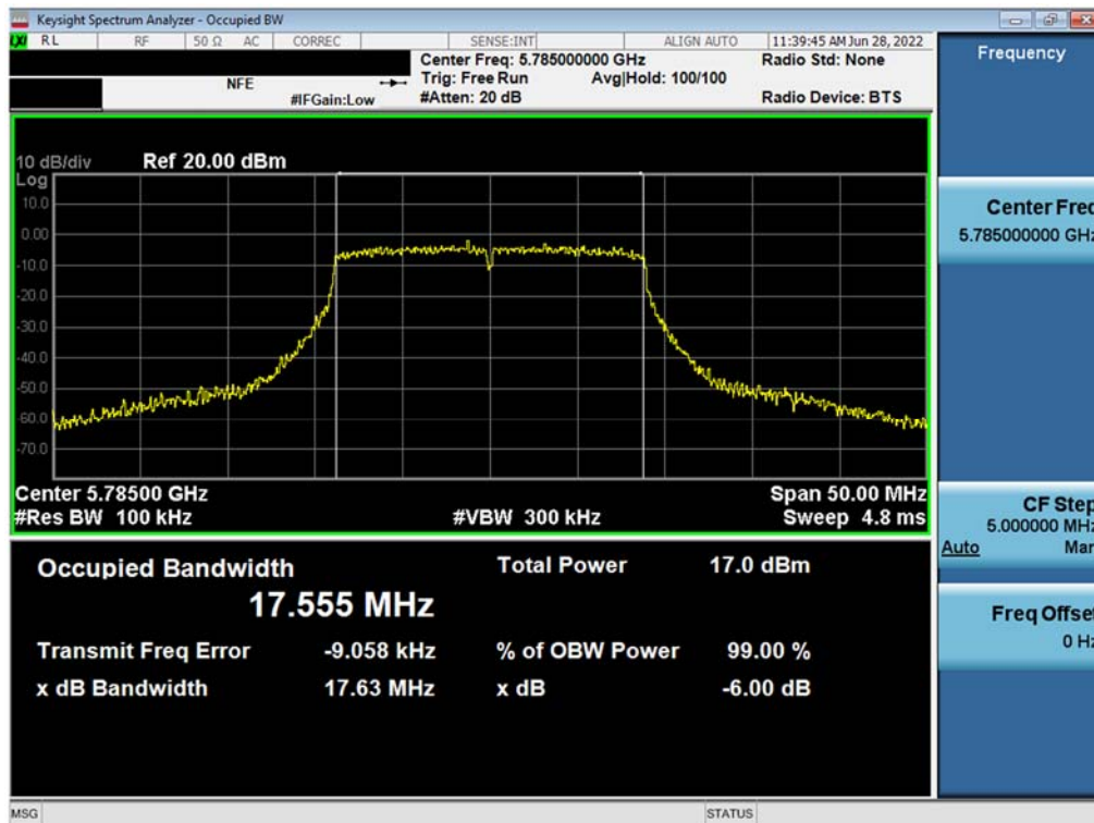
Plot 7-115. 6dB Bandwidth Plot MIMO ANT1 (802.11n – 20MHz BW (UNII Band 3) – Ch. 157)
