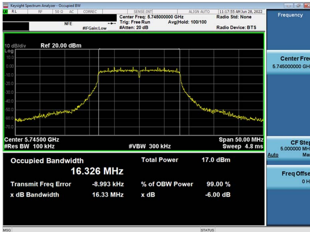
Plot 7-111. 6dB Bandwidth Plot MIMO ANT1 (802.11a (UNII Band 3) – Ch. 149)
