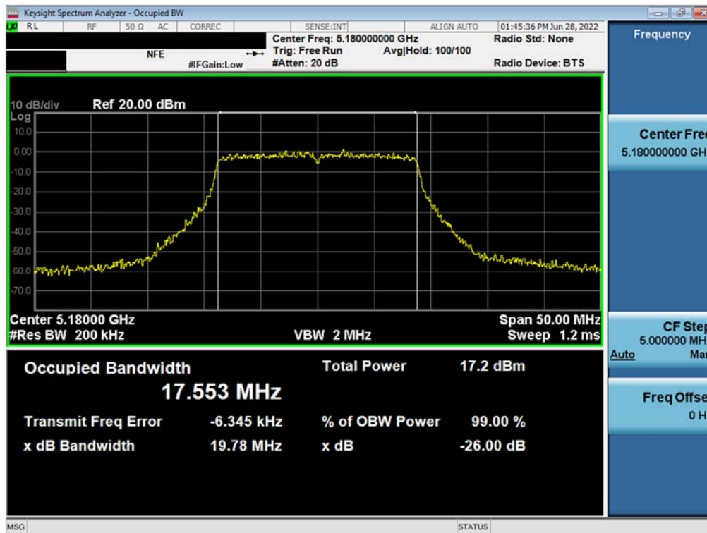
Plot 7-59. 26dB Bandwidth Plot MIMO ANT2 (802.11n – 20MHz BW (UNII Band 1) – Ch. 36)
