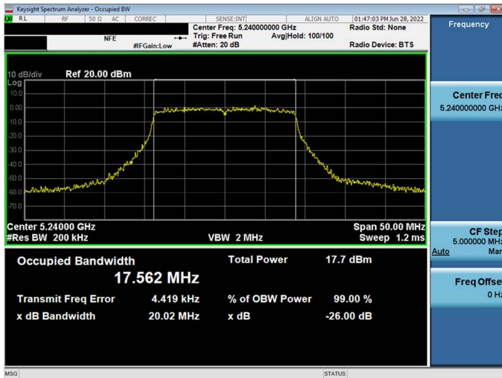
Plot 7-61. 26dB Bandwidth Plot MIMO ANT2 (802.11n – 20MHz BW (UNII Band 1) – Ch. 48)
