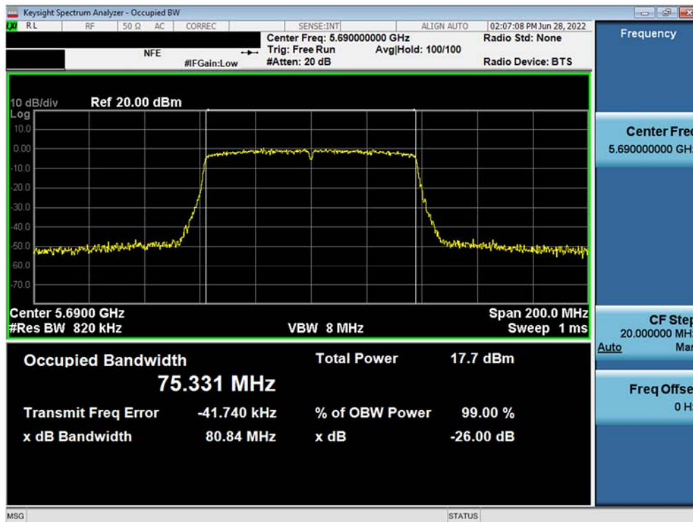
Plot 7-105. 26dB Bandwidth Plot MIMO ANT2 (802.11ac – 80MHz BW (UNII Band 2C) – Ch. 138)
