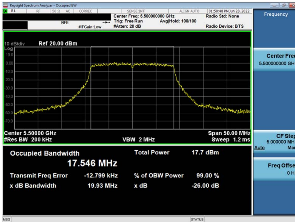
Plot 7-91. 26dB Bandwidth Plot MIMO ANT2 (802.11n – 20MHz BW (UNII Band 2C) – Ch. 100)
