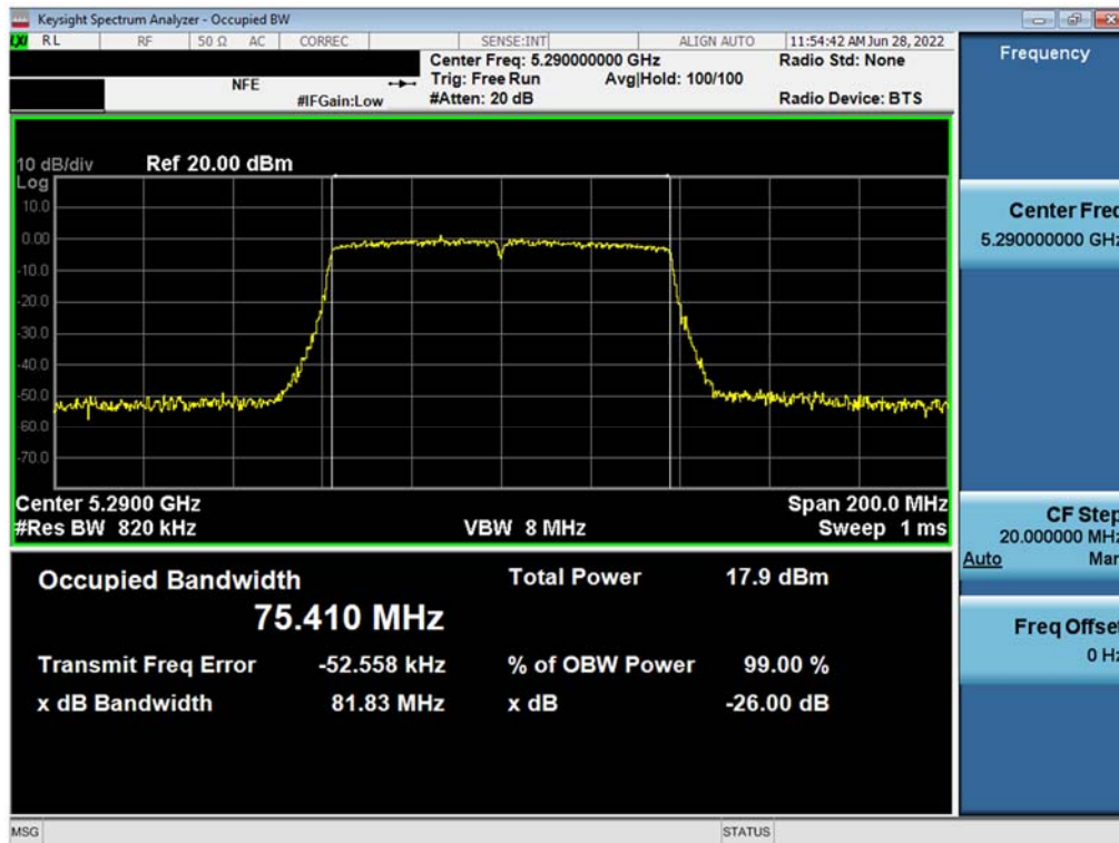
Plot 7-31. 26dB Bandwidth Plot MIMO ANT1 (802.11ac – 80MHz BW (UNII Band 2A) – Ch. 58)
