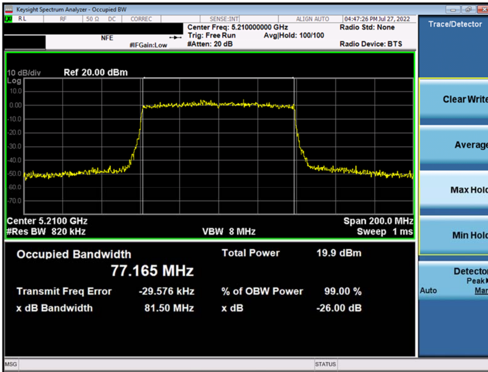
Plot 7-15. 26dB Bandwidth Plot MIMO ANT1 (802.11ax – 80MHz BW (UNII Band 1) – Ch. 42)
