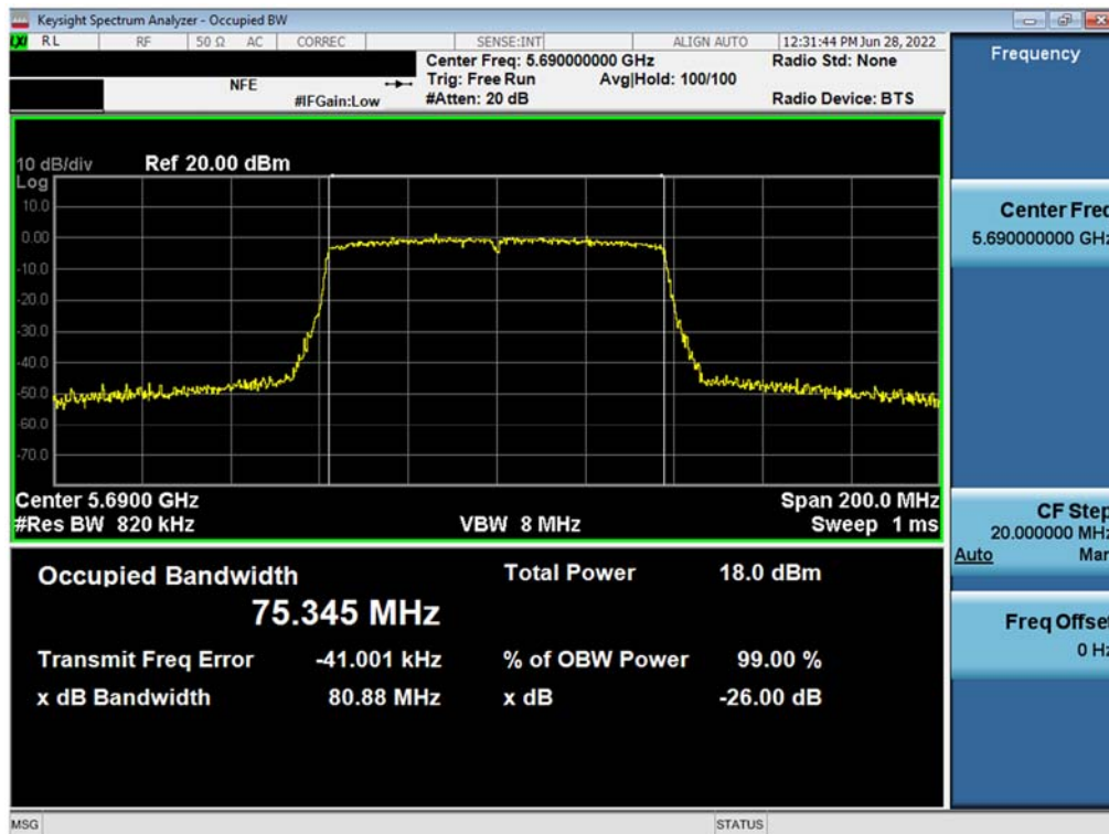
Plot 7-50. 26dB Bandwidth Plot MIMO ANT1 (802.11ac – 80MHz BW (UNII Band 2C) – Ch. 138)
