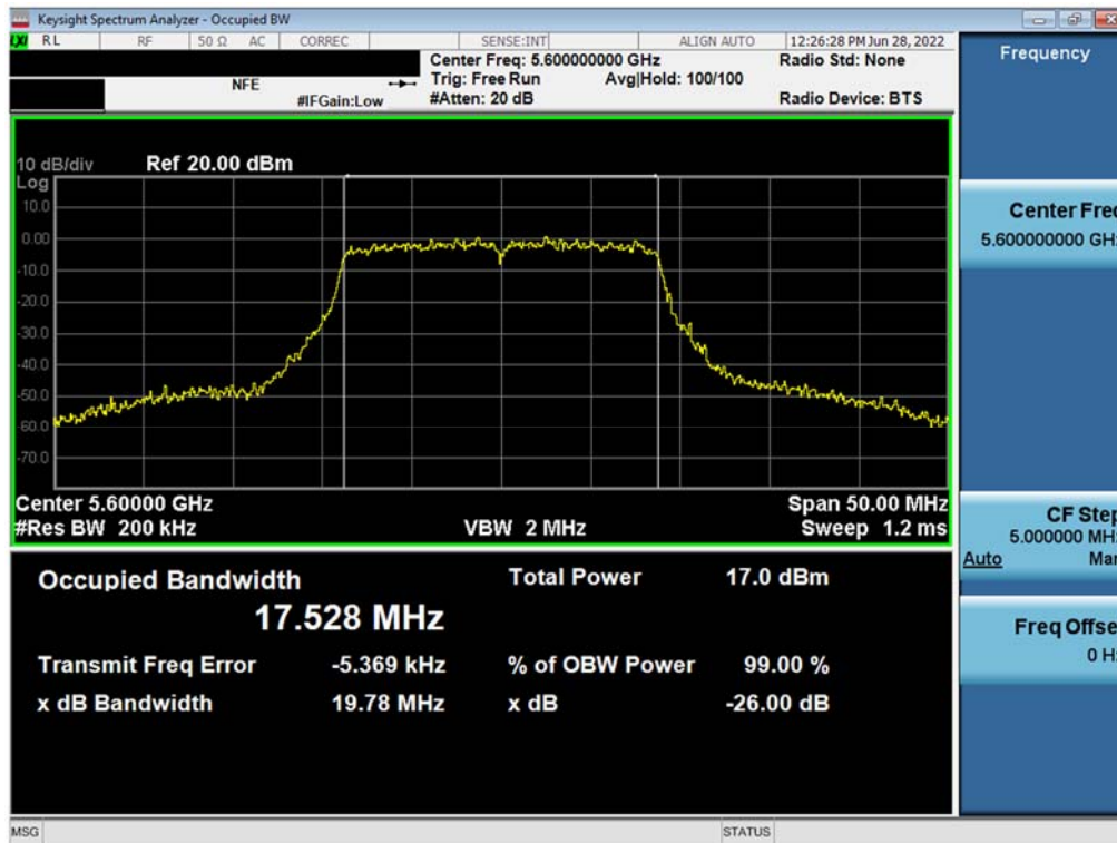
Plot 7-37. 26dB Bandwidth Plot MIMO ANT1 (802.11n – 20MHz BW (UNII Band 2C) – Ch. 120)
