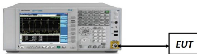
Figure 7-4. Test Instrument & Measurement Setup
