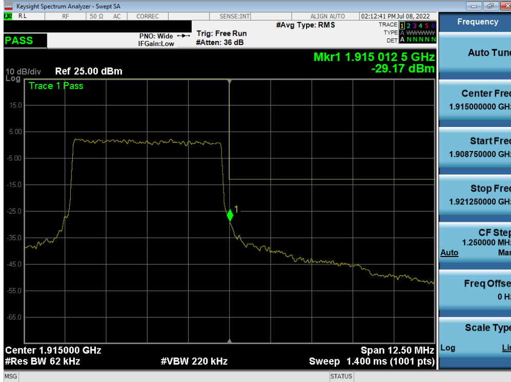
Plot 7-71. Upper Band Edge Plot (LTE Band 25 - 5MHz QPSK – Full RB)
