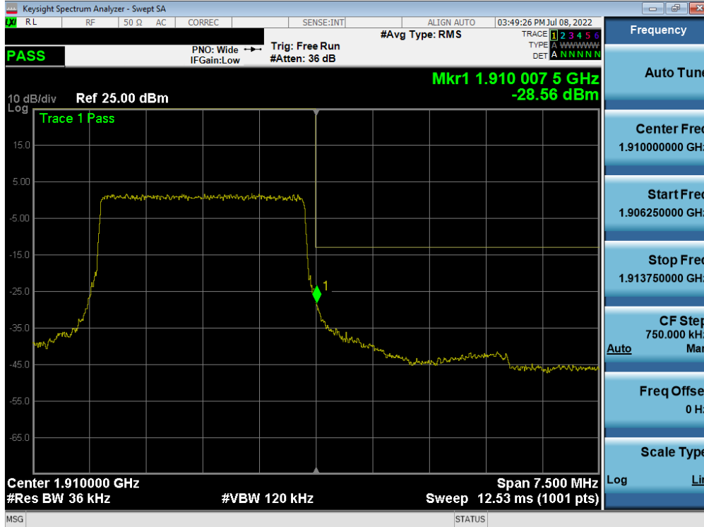
Plot 7-75. Upper Band Edge Plot (LTE Band 2 - 3MHz QPSK – Full RB)
