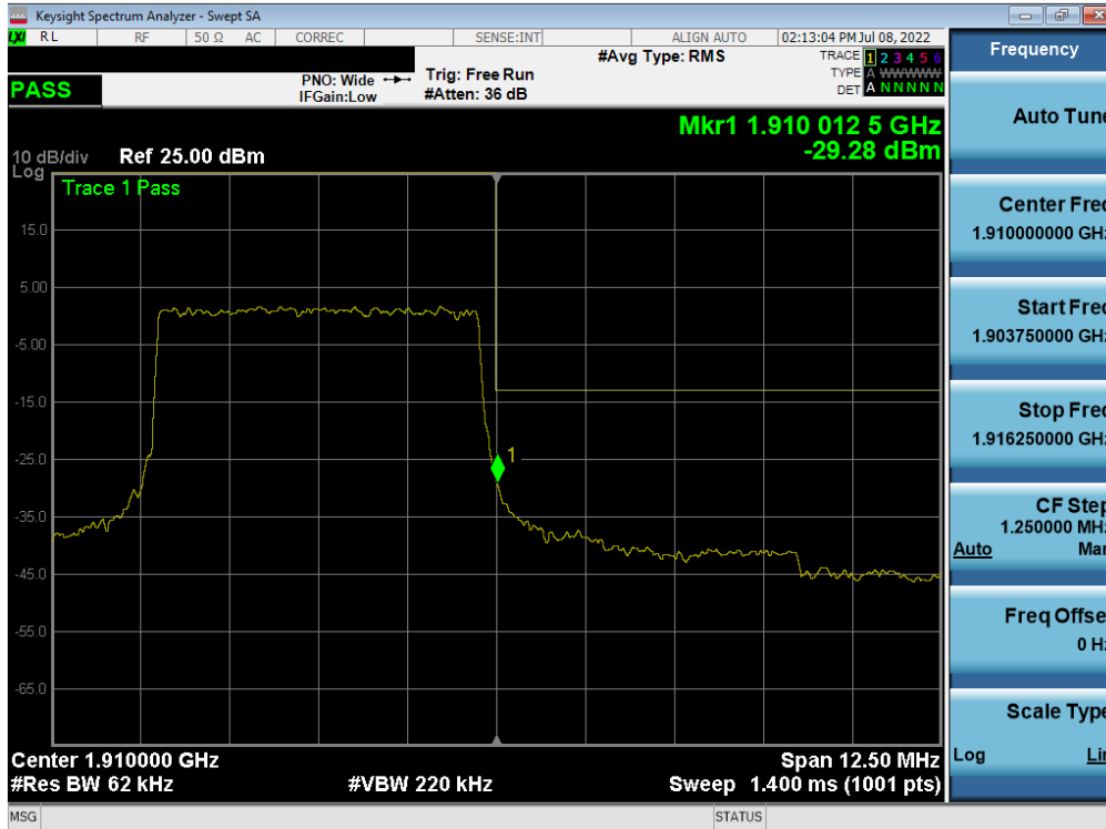
Plot 7-69. Upper Band Edge Plot (LTE Band 2 - 5MHz QPSK – Full RB)
