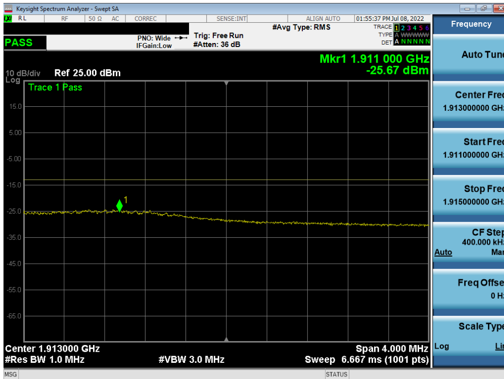
Plot 7-58. Extended Upper Band Edge Plot (LTE Band 2 - 15MHz QPSK – Full RB)
