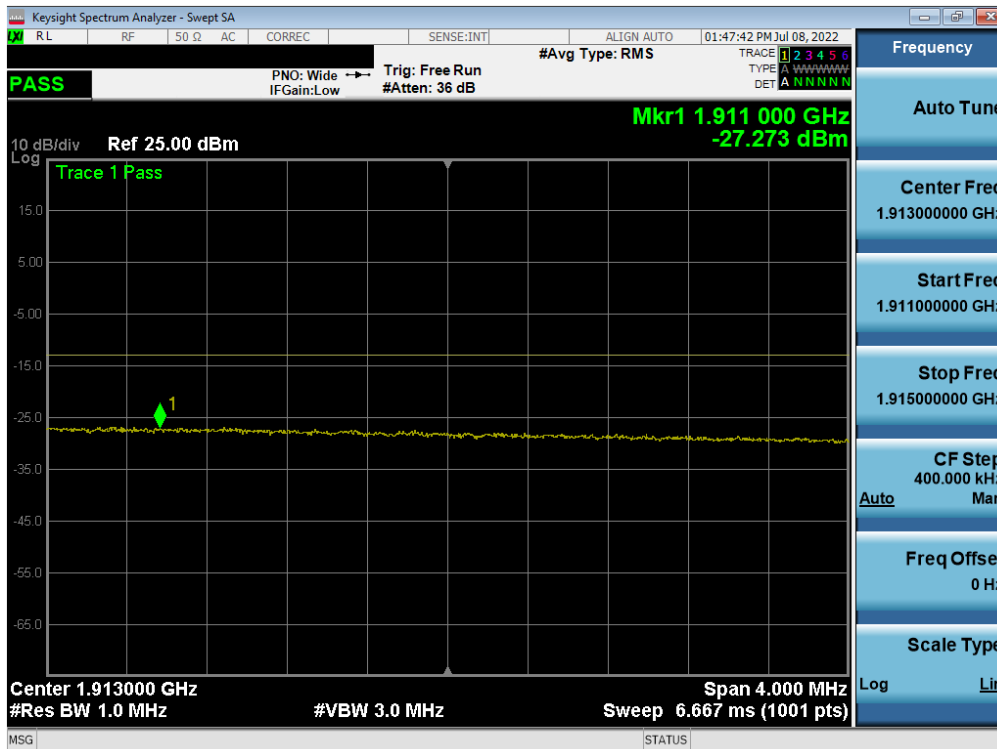
Plot 7-52. Extended Upper Band Edge Plot (LTE Band 2 - 20MHz QPSK – Full RB)
