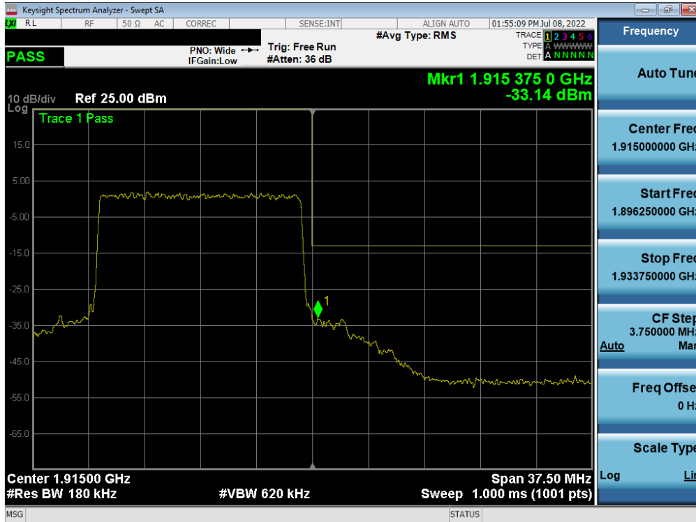
Plot 7-59. Upper Band Edge Plot (LTE Band 25 - 15MHz QPSK – Full RB)
