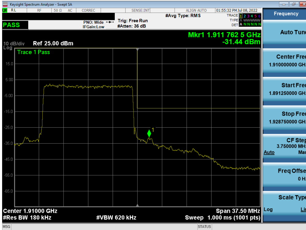
Plot 7-57. Upper Band Edge Plot (LTE Band 2 - 15MHz QPSK – Full RB)
