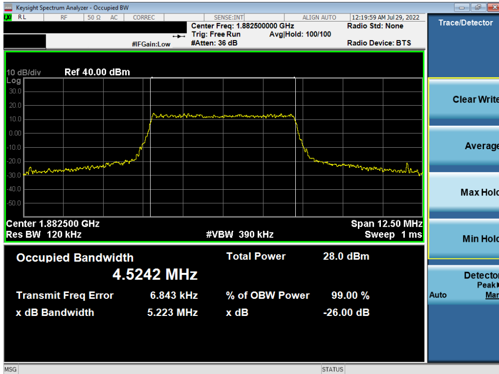
Plot 7-12. Occupied Bandwidth Plot (LTE Band 25/2 - 5MHz 64-QAM - Full RB)
