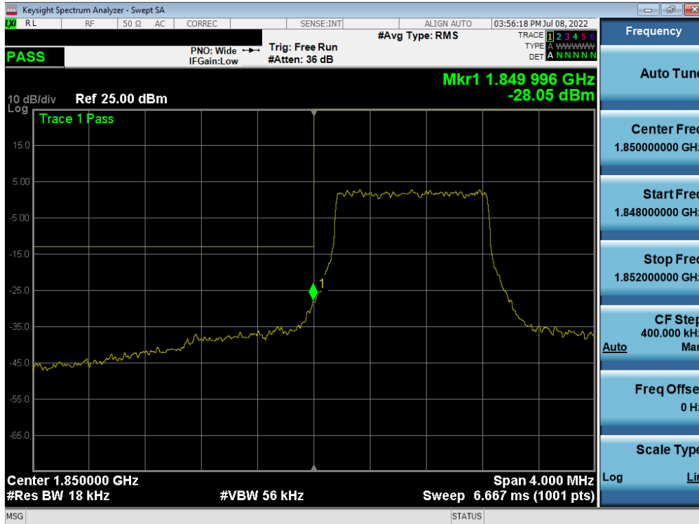
Plot 7-79. Lower Band Edge Plot (LTE Band 25/2 – 1.4MHz QPSK – Full RB)
