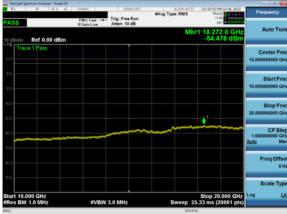
Plot 7-30. Conducted Spurious Plot (LTE Band 25/2 - 20MHz QPSK - 1RB - High Channel)
