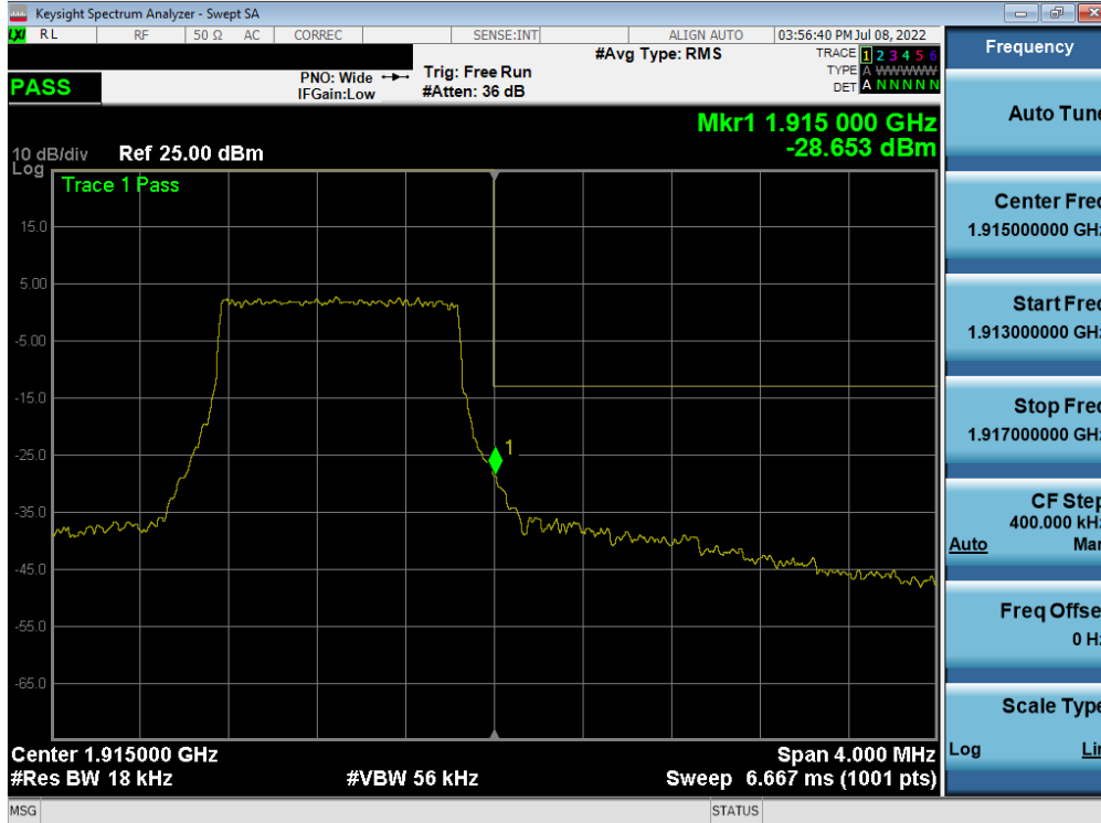
Plot 7-83. Upper Band Edge Plot (LTE Band 25 – 1.4MHz QPSK – Full RB)
