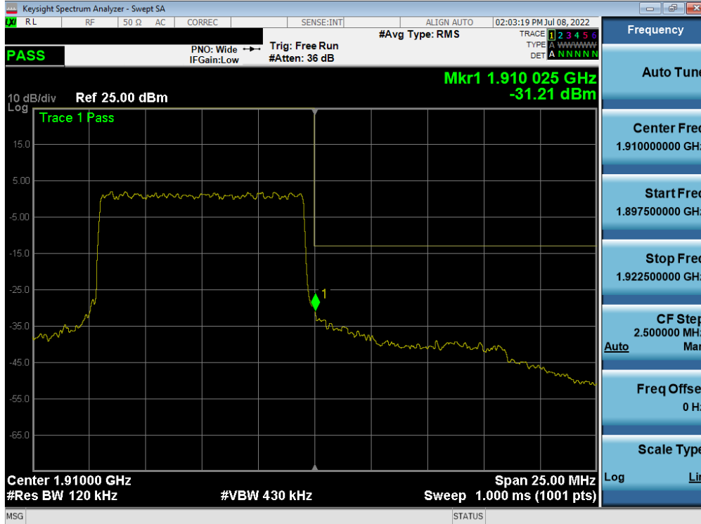
Plot 7-63. Upper Band Edge Plot (LTE Band 2 - 10MHz QPSK – Full RB)
