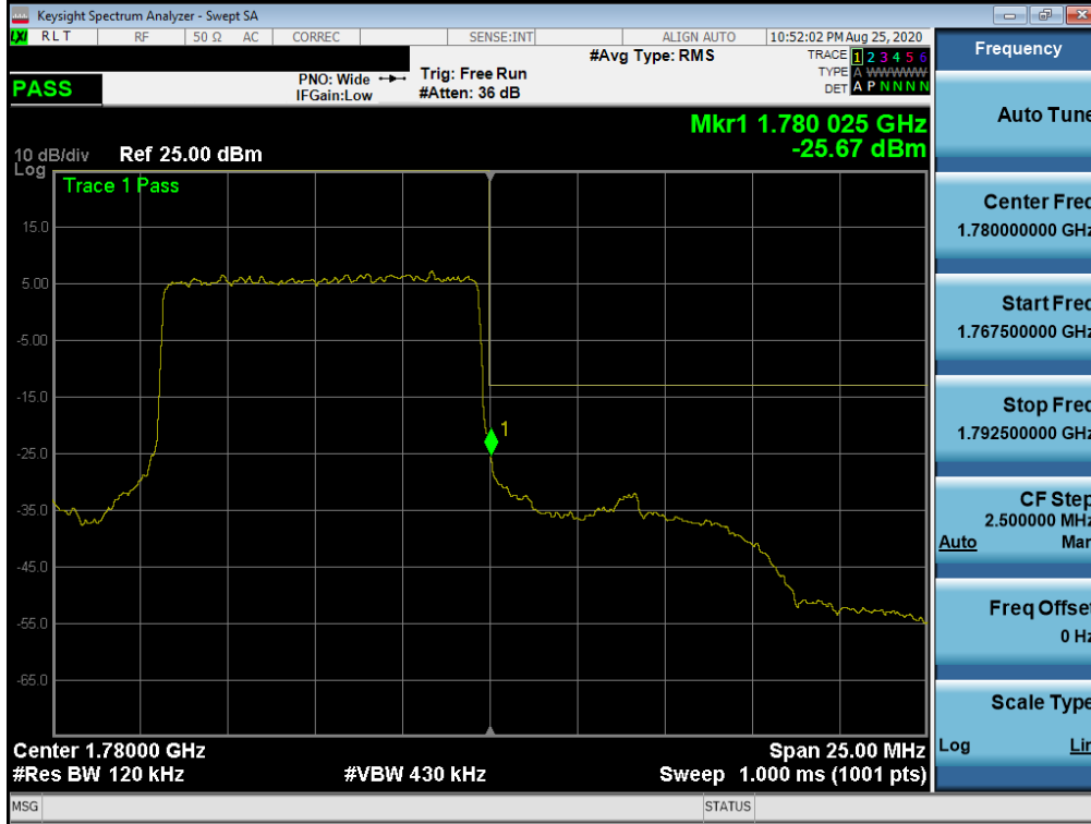
Plot 7-122. Upper Band Edge Plot (NR Band n66 – 10.0MHz - Full RB)
