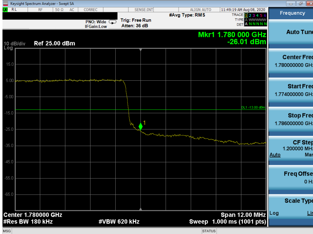
Plot 7-86. Upper Band Edge Plot (LTE Band 66 - 15MHz QPSK – Full RB Configuration)
