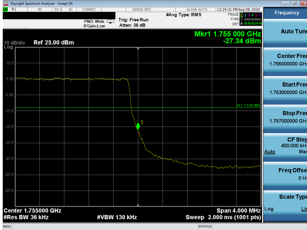
Plot 7-102. Upper Band Edge Plot (LTE Band 4 - 3MHz QPSK – Full RB Configuration)
