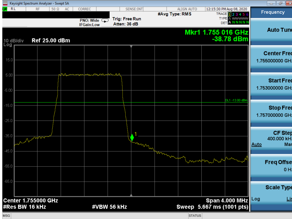
Plot 7-108. Upper Band Edge Plot (LTE Band 4 – 1.4MHz QPSK – Full RB Configuration)
