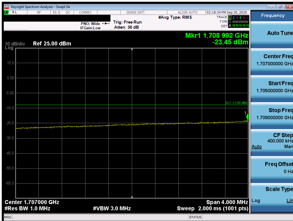
Plot 7-83. Lower Extended Band Edge Plot (LTE Band 66/4 - 15MHz QPSK – Full RB Configuration)
