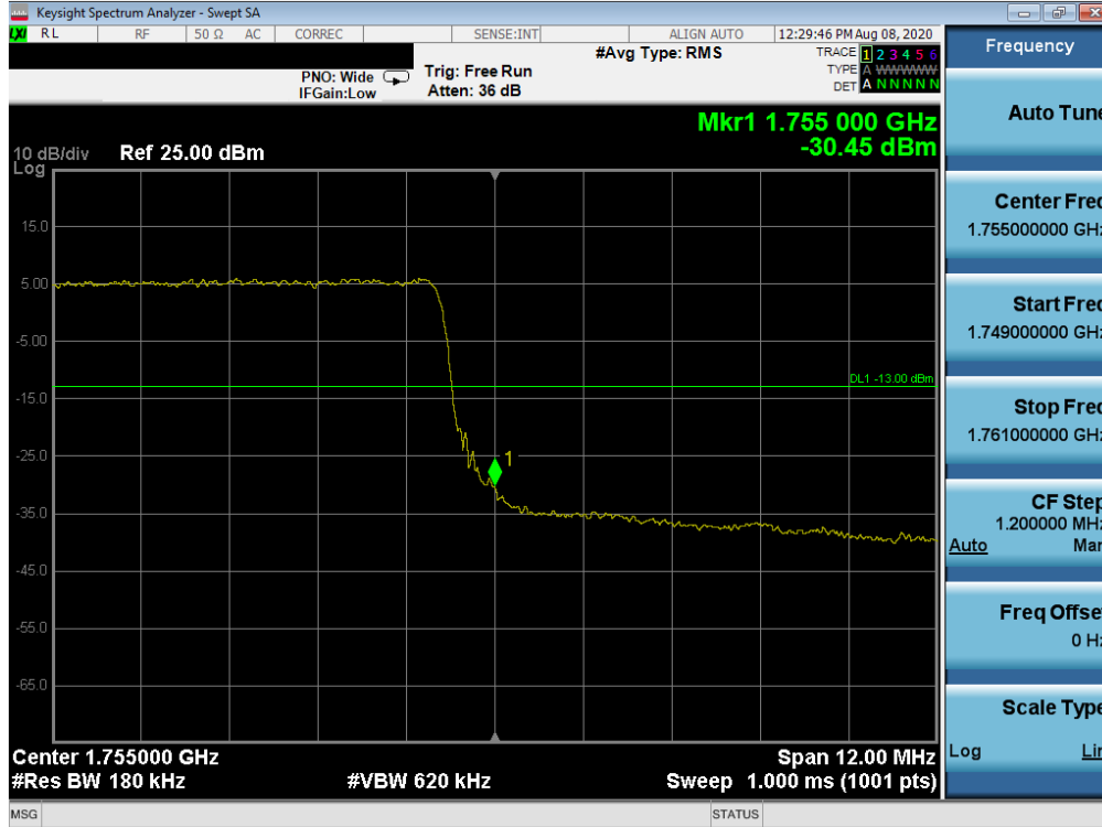
Plot 7-84. Upper Band Edge Plot (LTE Band 4 - 15MHz QPSK – Full RB Configuration)
