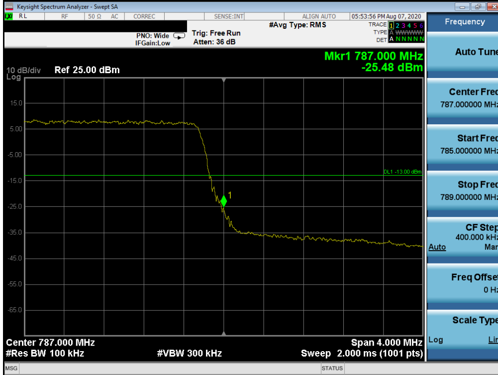
Plot 7-70. Upper Band Edge Plot (LTE Band 13 - 5MHz QPSK – Full RB Configuration)
