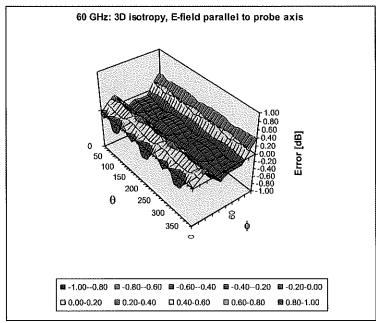
Probe isotropy for  $E_{tot}$ : probe rotated  $\phi = 0^\circ$  to 360°, tilted from field propagation direction  $\vec{k}$  Parallel to the field propagation ( $\psi = 0^\circ - 90^\circ$ ) at 30 GHz: deviation within  $\pm$  0.34 dB Parallel to the field propagation ( $\psi = 0^\circ - 90^\circ$ ) at 60 GHz: deviation within  $\pm$  0.37 dB
