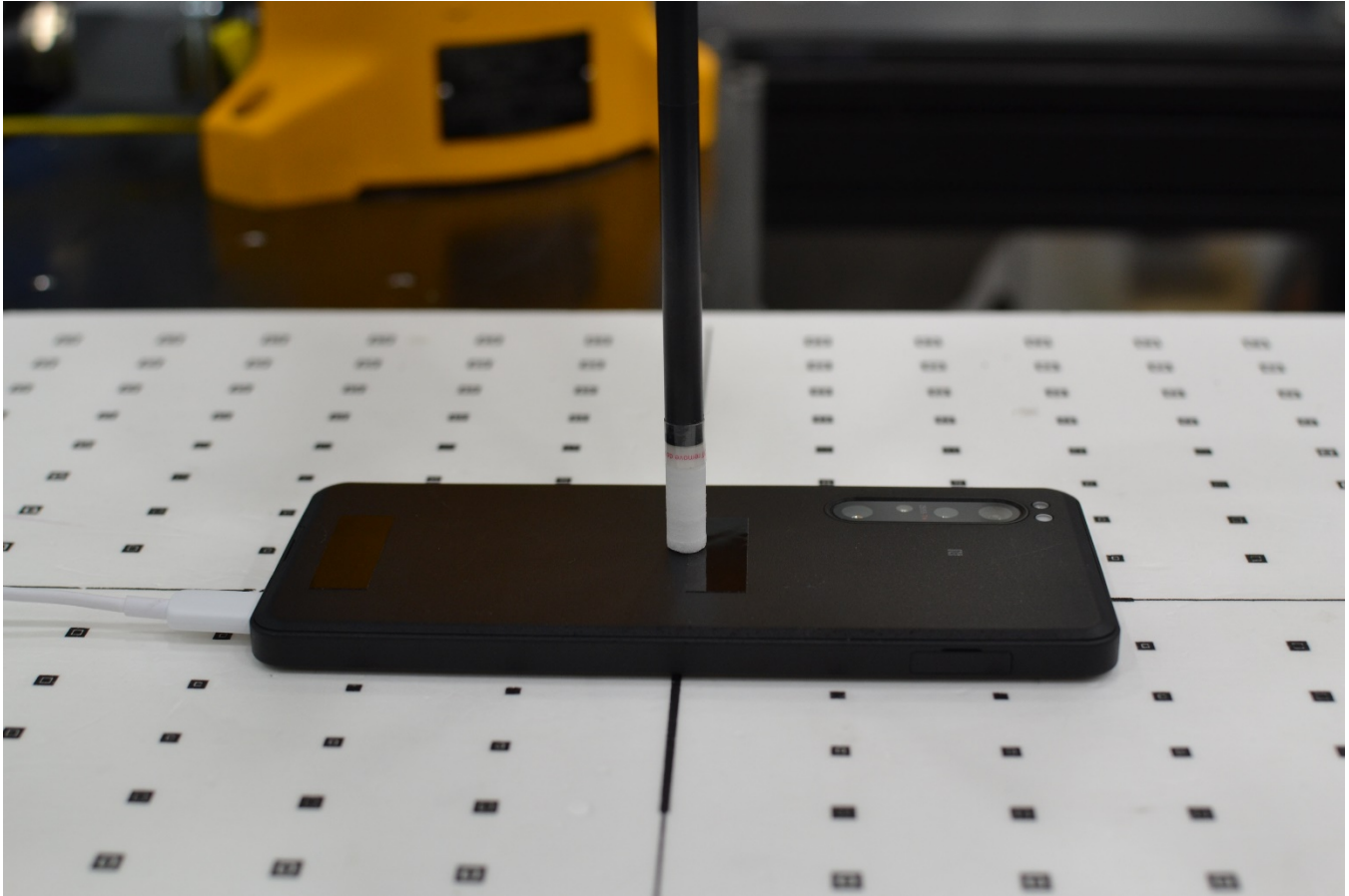
Figure D-3 Near Field Power Density Test Setup Photo – Back Side at 2 mm
