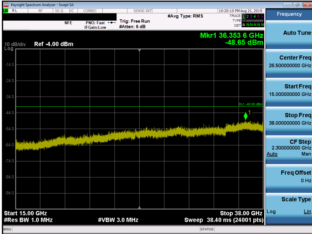
Plot 7-27. Conducted Spurious Plot (LTE Band 48 - 20.0MHz QPSK - RB Size 1, RB Offset 0 - High Channel)
