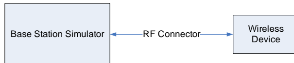
Figure 9-1 Power Measurement Setup
