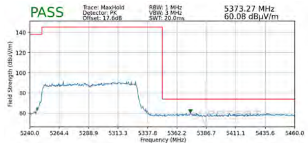
Plot 7-291. Radiated Upper Band Edge Plot SISO ANT2 (Peak – UNII Band 2A – 996 Tones)
