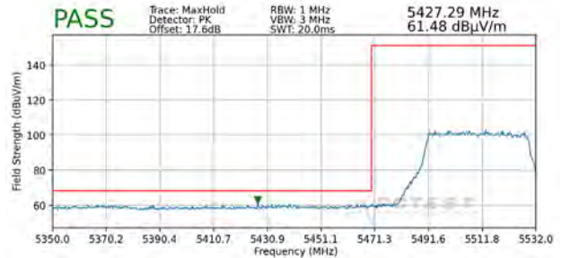
Plot 7-307. Radiated Lower Band Edge Plot MIMO (Peak – UNII Band 2C – 484 Tones)
